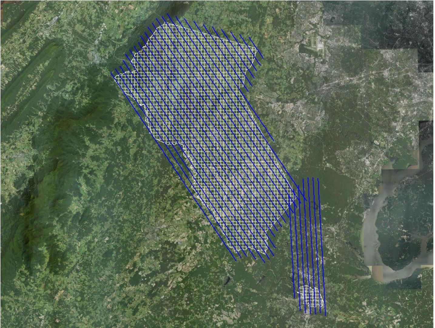
Figure 1: Tile Index and Trajectories As-Flown
