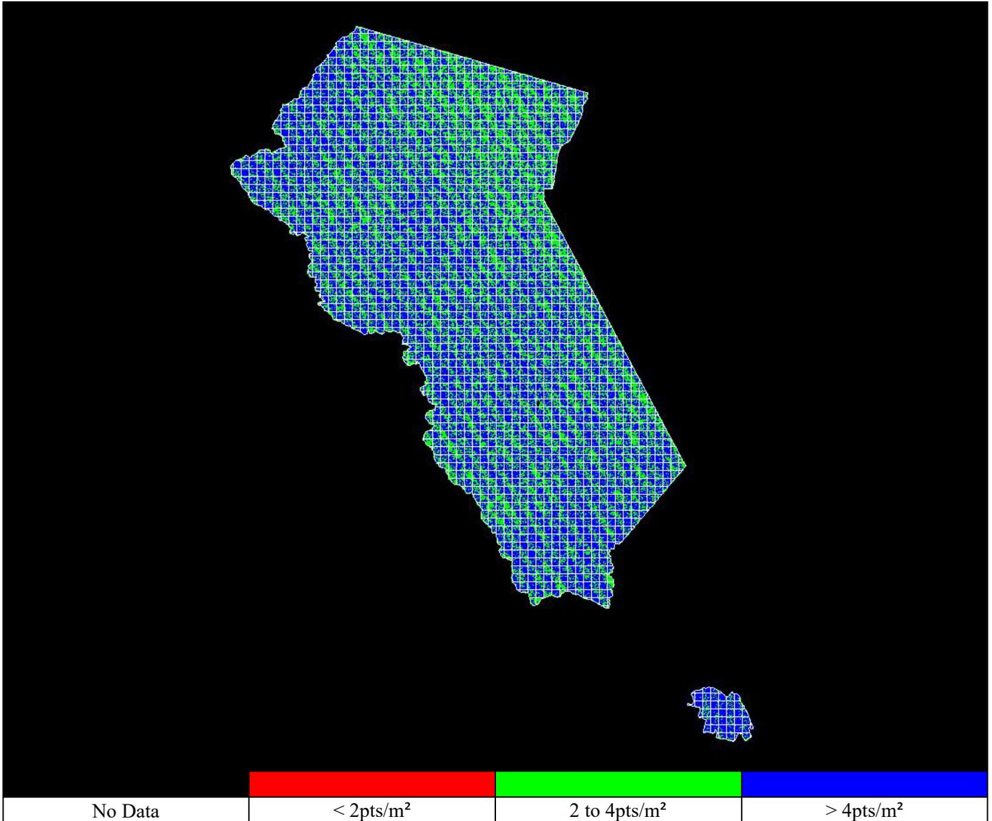
Figure 4: Point Cloud Density, of all points and all returns, no noise and no withheld points.
