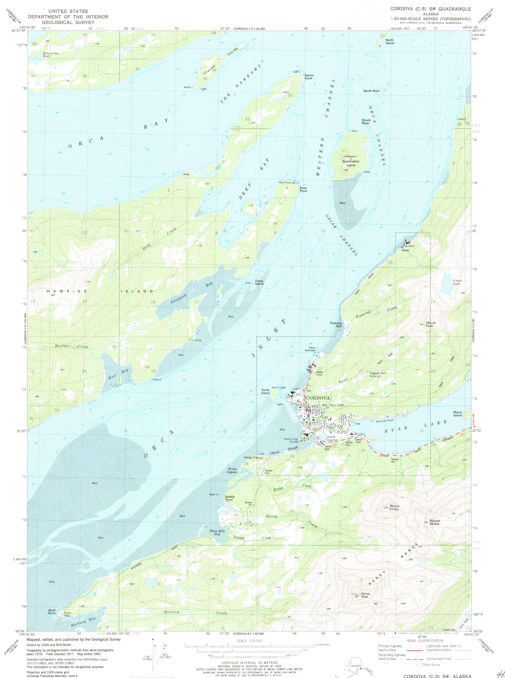
Universal Transverse Mercator, zone 6 10,000-foot grid ticks based on Alaska coordinate system, zone 3. 1927 North American datum To place on the predicted North American Datum 1983 move the projection lines 60 meters north and 112 meters east as shown by dashed corner ticks
