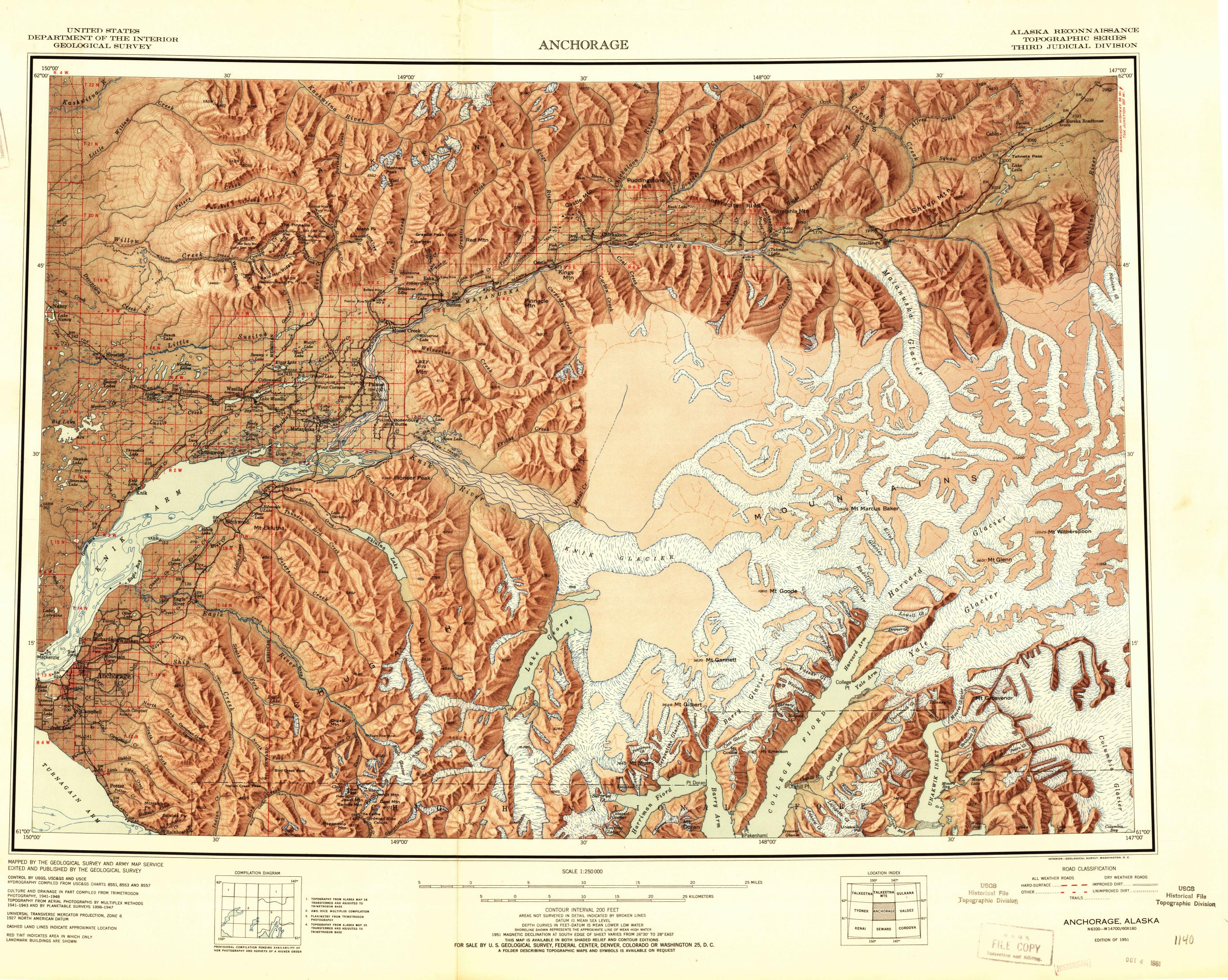
CONTROL BY USGS, USC&GS AND USCE HYDROGRAPHY COMPILED FROM USC&GS CHARTS 8551, 8553 AND 8557 CULTURE AND DRAINAGE IN PART COMPILED FROM TRIMETROGON PHOTOGRAPHY, 1941–1948 TOPOGRAPHY FROM AERIAL PHOTOGRAPHS BY MULTIPLEX METHODS 1941–1943 AND BY PLANETABLE SURVEYS 1898–1947 UNIVERSAL TRANSVERSE MERCATOR PROJECTION, ZONE 6 DASHED LAND LINES INDICATE APPROXIMATE LOCATION
