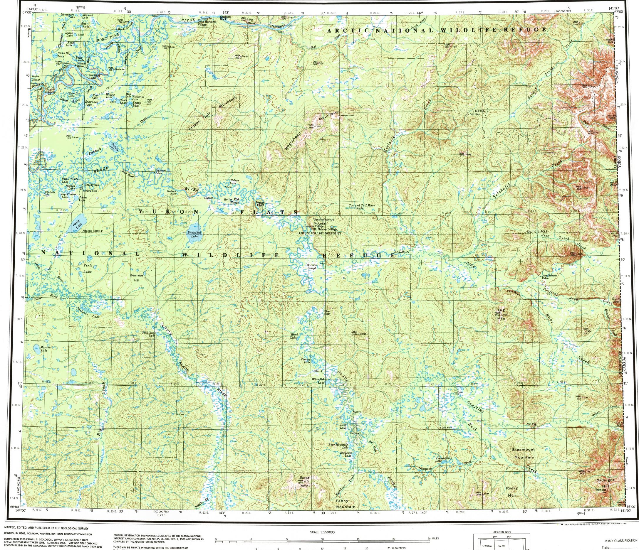
PROJECTION AND 10,000-METER GRID UNIVERSAL TRANSVERSE MERCATOR, ZONE 7 100,000-FOOT GRID TICKS BASED ON ALASKA COORDINATE SYSTEM, ZONE 2 1927 NORTH AMERICAN DATUM. TO PLACE ON THE PREDICTED NORTH AMERICAN DATUM 1983 MOVE THE PROJECTION LINES 35 METERS NORTH AND 111 METERS EAST
