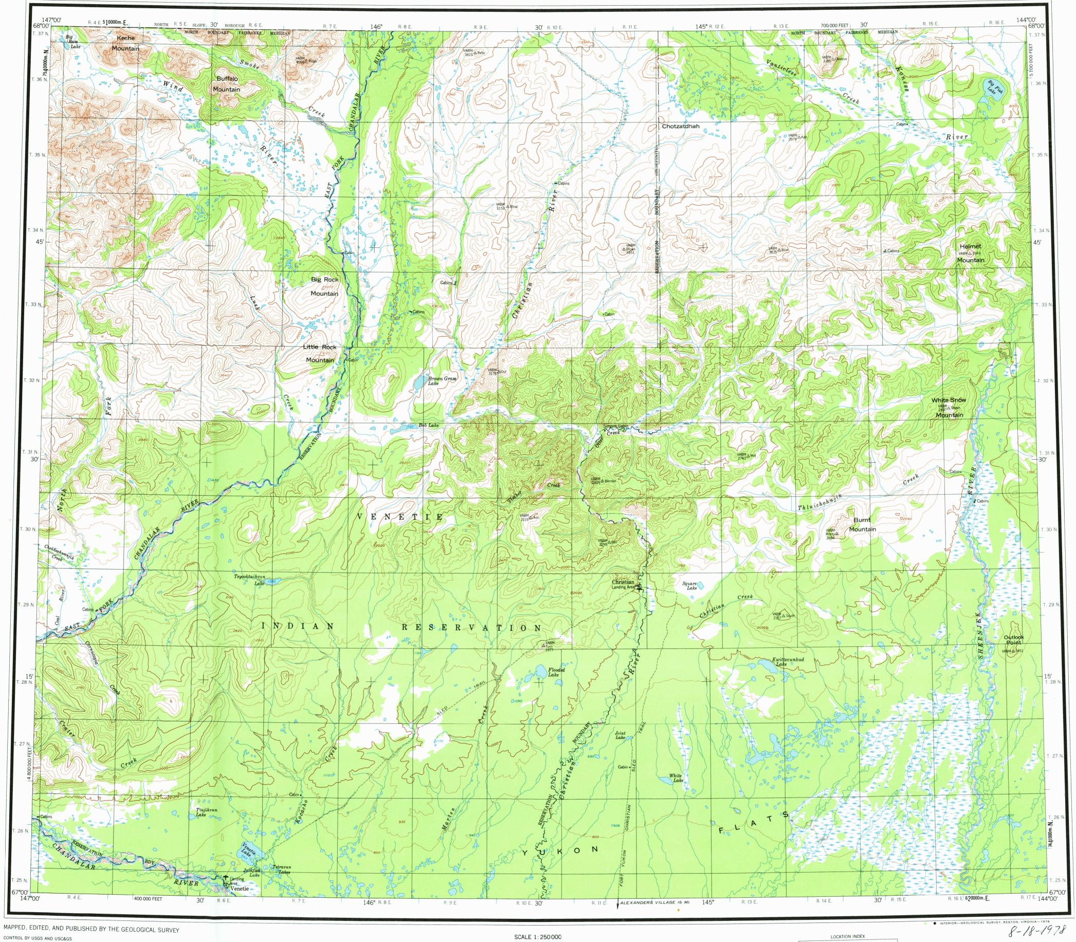
TOPOGRAPHY BY PHOTOGRAMMETRIC METHODS FROM AERIAL PHOTOGRAPHS TAKEN 1955. FIELD ANNOTATED 1956, MAP NOT FIELD CHECKED UNIVERSAL TRANSVERSE MERCATOR PROJECTION, 1927 NORTH AMERICAN DATUM 100 000-FOOT GRID BASED ON ALASKA COORDINATE SYSTEM, ZONE 3 10 000-METER UNIVERSAL TRANSVERSE MERCATOR GRID TICKS, ZONE 6, SHOWN IN BLUE LAND LINES REPRESENT UNSURVEYED AND UNMARKED LOCATIONS PREDETERMINED BY THE BUREAU OF LAND MANAGEMENT FOLIOS F-1 AND F-2, FAIRBANKS MERIDIAN
