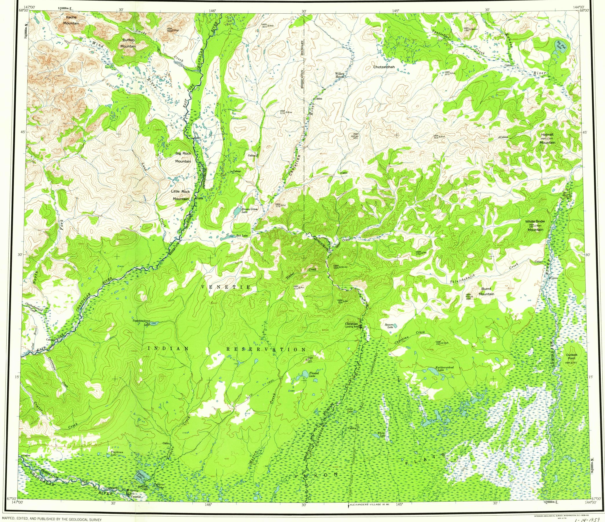
CONTROL BY USGS AND USC&GS TOPOGRAPHY FROM AERIAL PHOTOGRAPHS BY PHOTOGRAMMETRIC METHODS 1957. AERIAL PHOTOGRAPHS TAKEN 1955, FIELD ANNOTATED 1956. MAP NOT FIELD CHECKED UNIVERSAL TRANSVERSE MERCATOR PROJECTION 1927 NORTH AMERICAN DATUM 10,000-METER UNIVERSAL TRANSVERSE MERCATOR GRID TICKS, ZONE 6, SHOWN IN BLUE UNCHECKED ELEVATIONS ARE SHOWN IN BROWN AND BLUE
