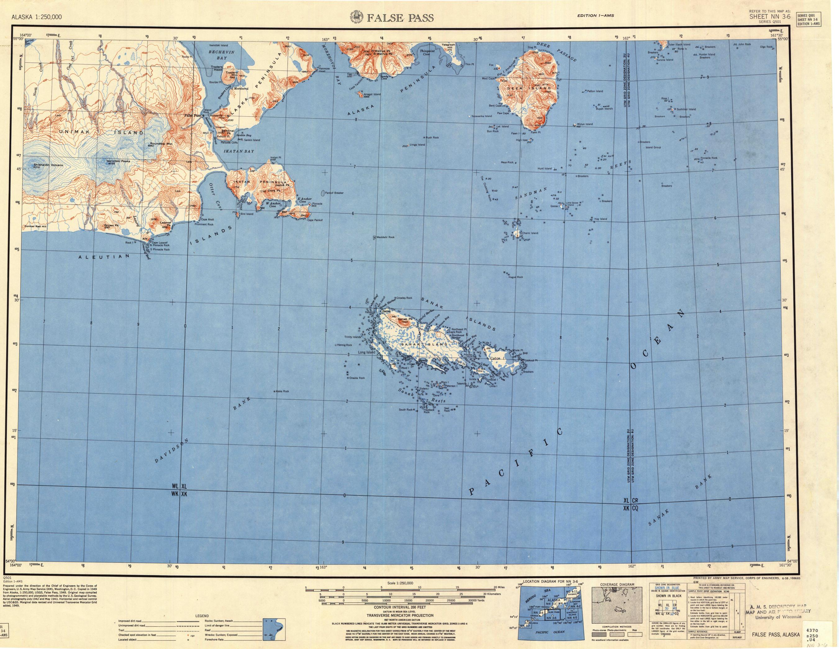
from Alaska, 1:250,000, USGS, False Pass, 1949. Original map compiled by photogrammetric and planetable methods by the U.S. Geological Survey. Aerial photography July 1942 and May 1943. Horizontal and vertical control
