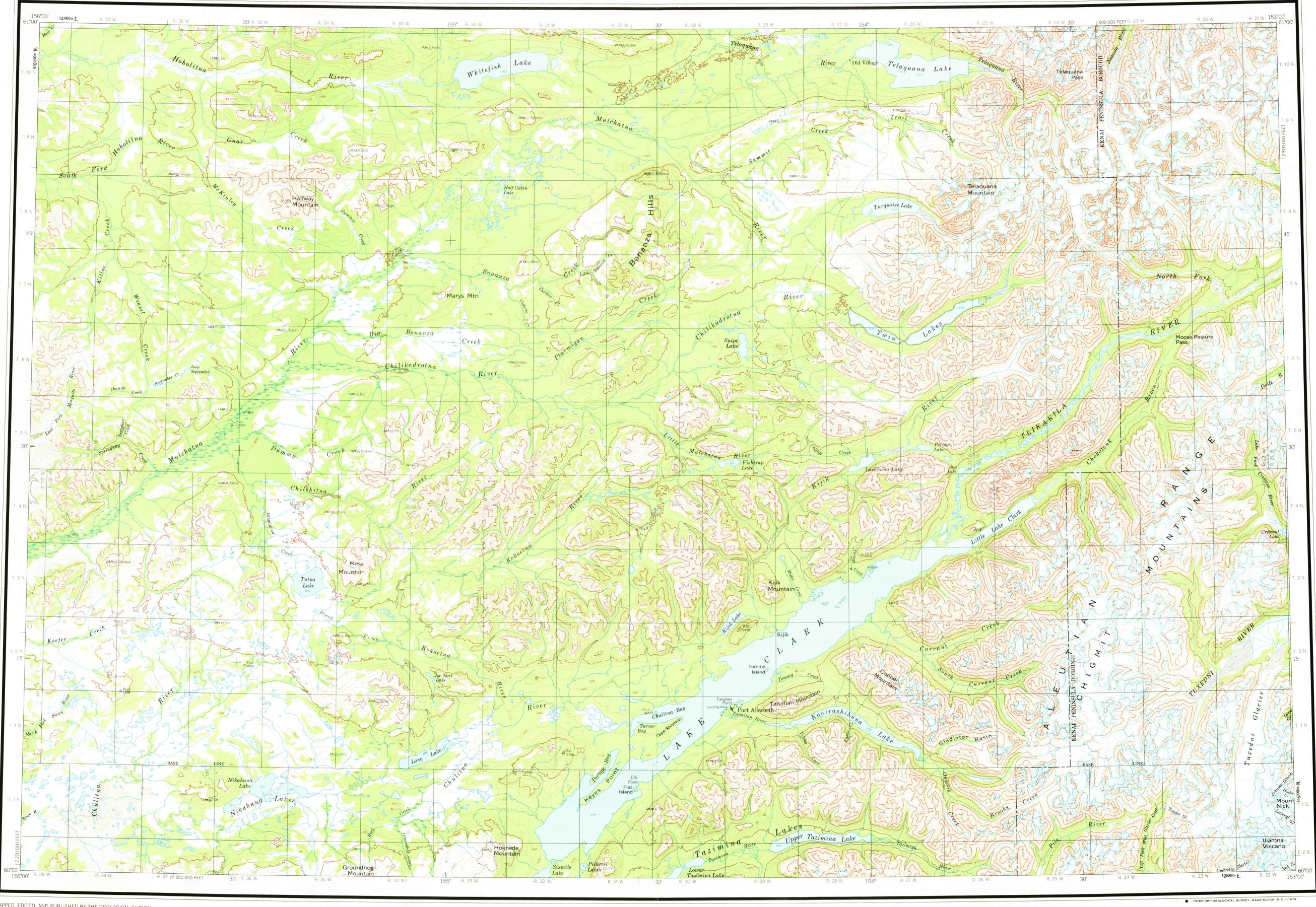
MAPPED, EDITED, AND PUBLISHED BY THE GEOLOGICAL SURVEY CONTROL BY USGS, USC&GS, AND USCE COMPILED IN 1966 FROM U.S. GEOLOGICAL SURVEY 1:63 360-SCALE MAPS, AND FROM ARMY MAP SERVICE 1:50 000 SERIES MAPS, SURVEYED 1953-1958 MAP NOT FIELD CHECKED UNIVERSAL TRANSVERSE MERCATOR PROJECTION. 1927 NORTH AMERICAN DATUM 100,000-FOOT GRID BASED ON ALASKA COORDINATE SYSTEM, ZONE 5 10,000-METER UNIVERSAL TRANSVERSE MERCATOR GRID TICKS, ZONE 5, SHOWN IN BLUE
