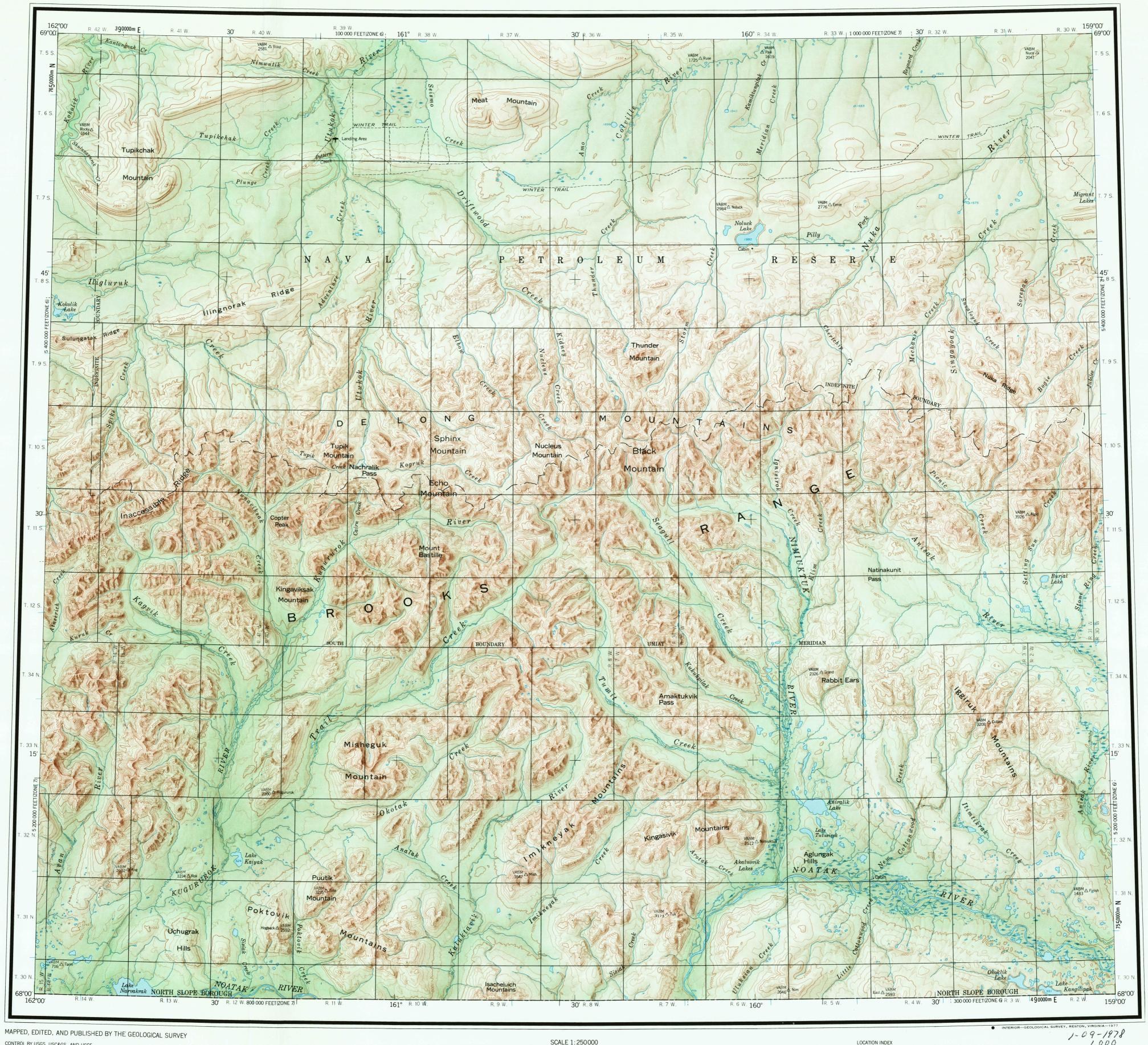
CONTROL BY USGS, USC&GS, AND USCE TOPOGRAPHY BY PHOTOGRAMMETRIC METHODS FROM AERIAL PHOTOGRAPHS TAKEN 1955-1956, AND FROM ARMY MAP SERVICE 1:50, 000 SERIES MAPS, SURVEYED 1958. FIELD ANNOTATED 1956. MAP NOT FIELD CHECKED UNIVERSAL TRANSVERSE MERCATOR PROJECTION, 1927 NORTH AMERICAN DATUM 100,000-F00T GRIDS BASED ON ALASKA COORDINATE SYSTEM, ZONES 7 AND 6 10,000-METER UNIVERSAL TRANSVERSE MERCATOR GRID TICKS, ZONE 4, SHOWN IN BLUE
