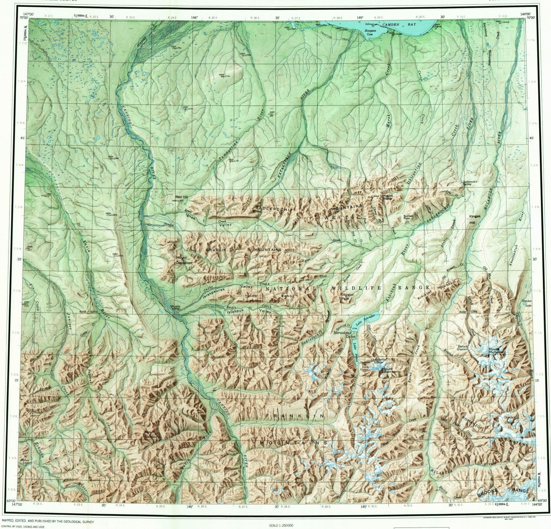
CONTROL BY USGS, USC&GS AND USCE TOPOGRAPHY FROM AERIAL PHOTOGRAPHS BY PHOTOGRAMMETRIC METHODS 1957, AND FROM ARMY MAP SERVICE 1:50,000 SERIES MAPS, SURVEYED 1955. AERIAL PHOTOGRAPHS TAKEN 1956, FIELD ANNOTATED 1956 MAP NOT FIELD CHECKED SELECTED HYDROGRAPHIC DATA COMPILED FROM USC & GS CHART 9475 (1956) THIS INFORMATION IS NOT INTENDED FOR NAVIGATIONAL PURPOSES
