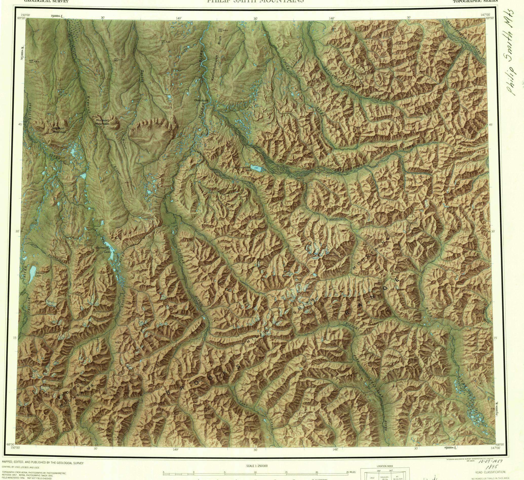
CONTROL BY USGS, USC&GS, AND USCE TOPOGRAPHY FROM AERIAL PHOTOGRAPHS BY PHOTOGRAMMETRIC METHODS 1957. AERIAL PHOTOGRAPHS TAKEN 1955, FIELD ANNOTATED 1956. MAP NOT FIELD CHECKED
