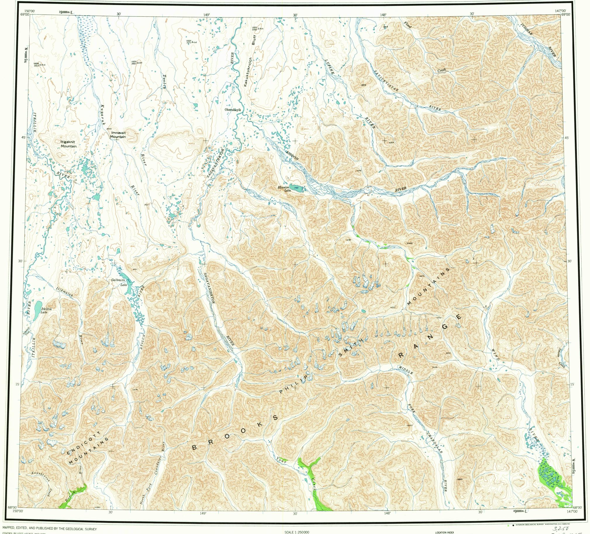
CONTROL BY USGS, USC&GS, AND USCE TOPOGRAPHY FROM AERIAL PHOTOGRAPHS BY PHOTOGRAMMETRIC METHODS 1957. AERIAL PHOTOGRAPHS TAKEN 1955, FIELD ANNOTATED 1956. MAP NOT FIELD CHECKED UNIVERSAL TRANSVERSE MERCATOR PROJECTION 1927 NORTH AMERICAN DATUM 10,000-METER UNIVERSAL TRANSVERSE MERCATOR GRID TICKS, ZONE 6, SHOWN IN BLUE
