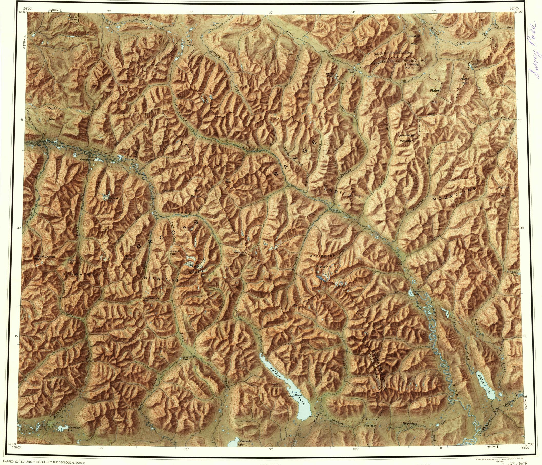
CONTROL BY USGS TOPOGRAPHY FROM AERIAL PHOTOGRAPHS BY PHOTOGRAMMETRIC METHODS 1957. AERIAL PHOTOGRAPHS TAKEN 1955, FIELD ANNOTATED 1956. MAP NOT FIELD CHECKED
