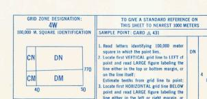
IGNORE the SMALLER figures of any grid number; these are for finding the full coordinates. Use ONLY the LARGER figure of the grid number; example: 7660000
