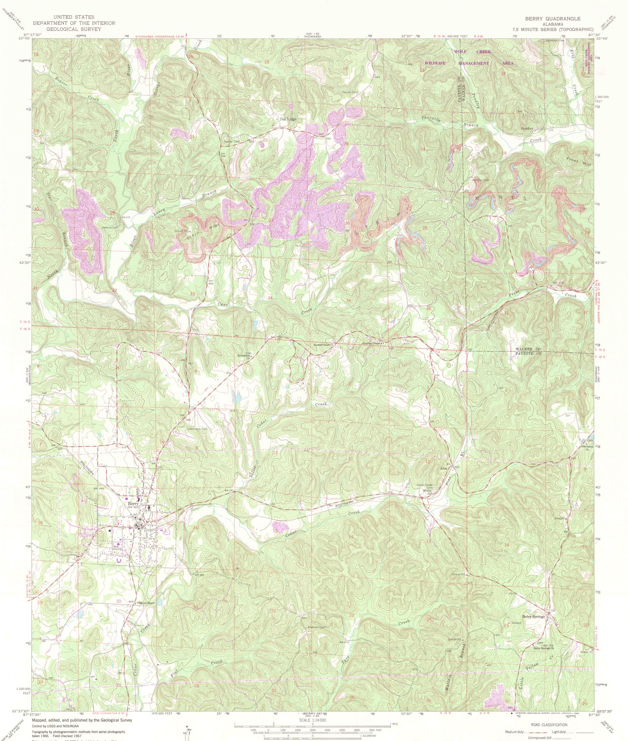
Polyconic projection. 10,000-foot grid ticks based on Alabama coordinate system, west zone. 1000-meter Universal Transverse Mercator grid ticks, zone 16, shown in blue. 1927 North American Datum. To place on the predicted North American Datum 1983 move the projection lines 10 meters south and 1 meter east as shown by dashed corner ticks
