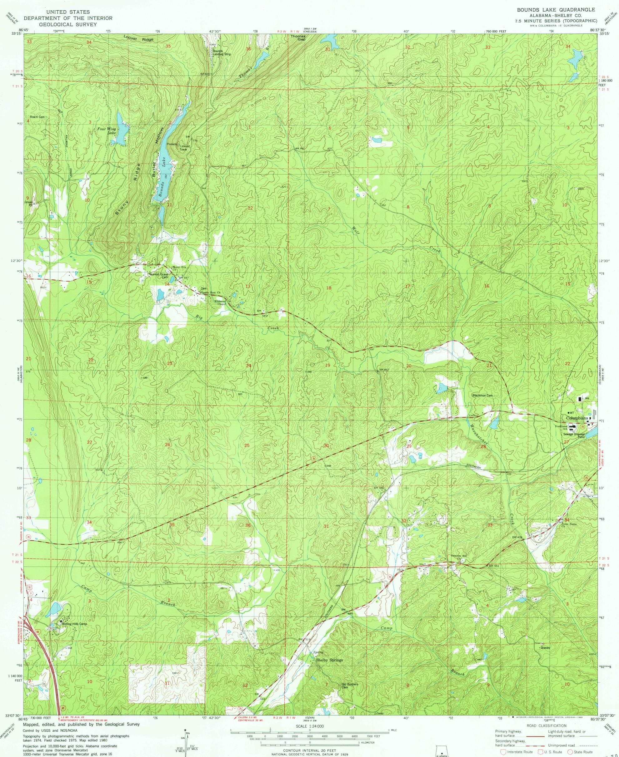
system, west zone (transverse Mercator) 1000-meter Universal Tranverse Mercator grid, zone 16 1927 North American Datum To place on the predicted North American Datum 1983 move the projection lines 10 meters south and 2 meters west as shown by dashed corner ticks
