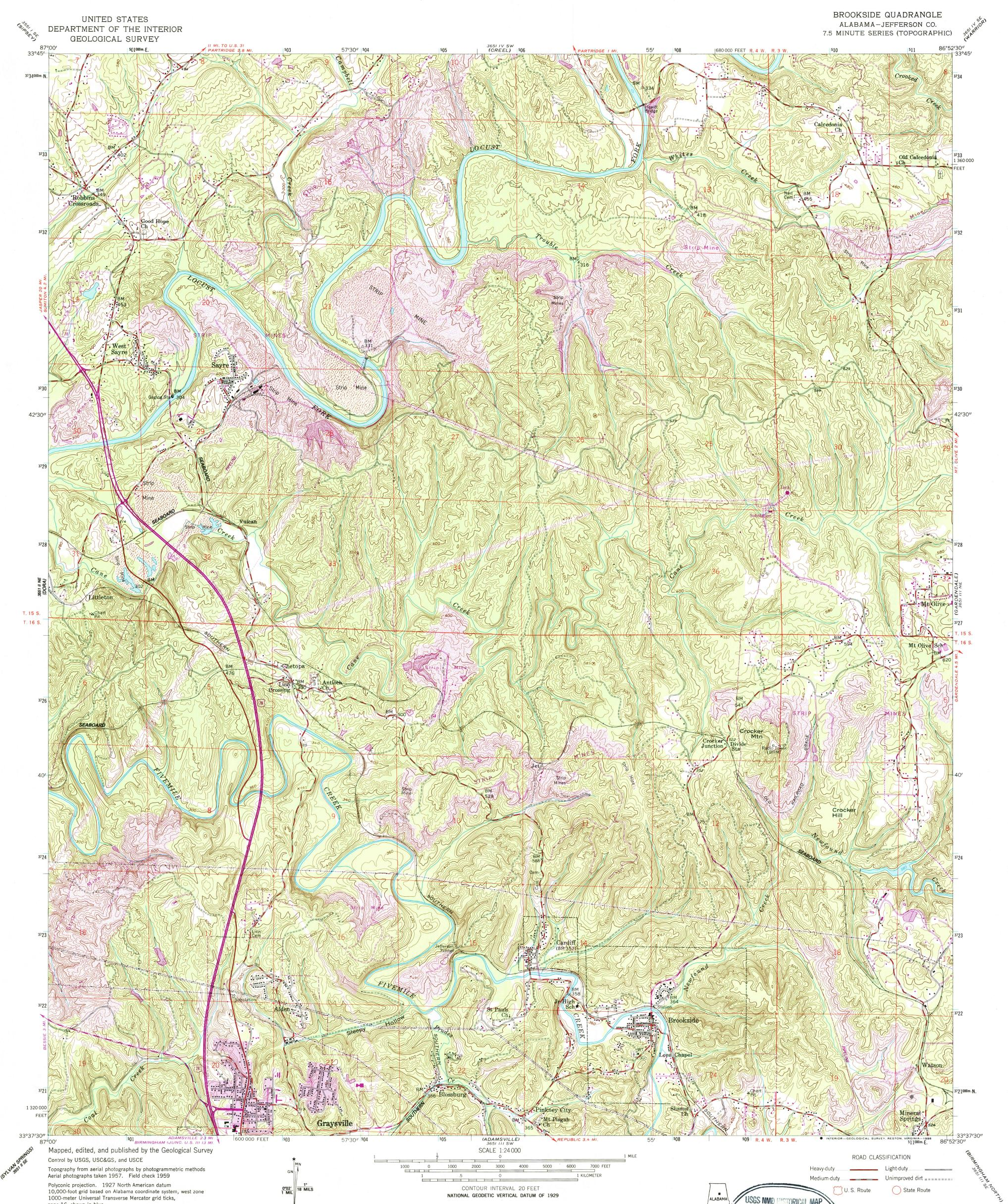
10,000-foot grid based on Alabama coordinate system, west zone 1000-meter Universal Transverse Mercator grid ticks, zone 16, shown in blue To place on the predicted North American Datum 1983, move the projection lines 9 meters north and 1 meter west as shown by dashed corner ticks
