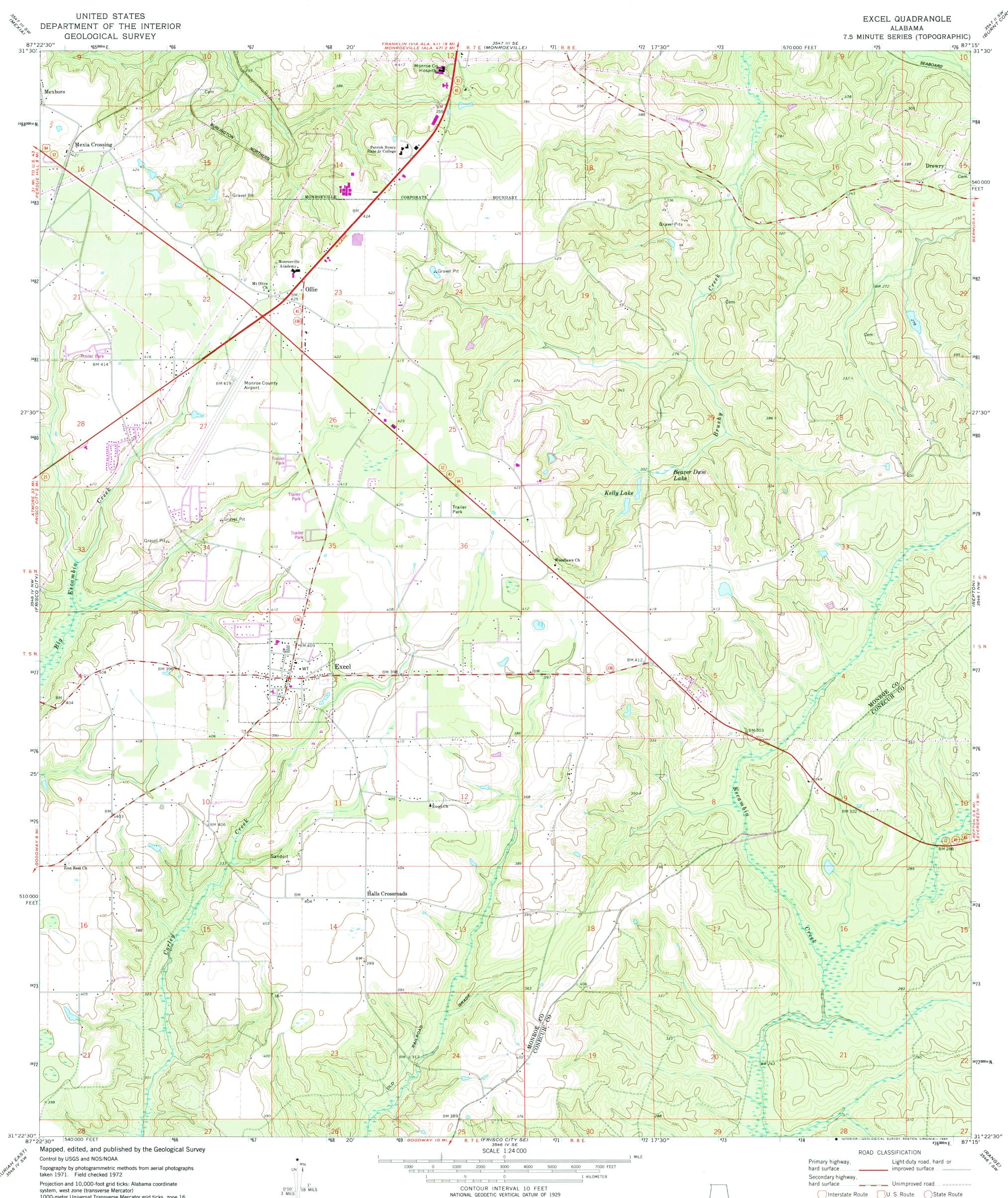
1000-meter Universal Transverse Mercator shown in blue 1927 North American Datum To place on the predicted North American Datum 1983 move the projection lines 15 meters south and 2 meters west as shown by dashed corner ticks
