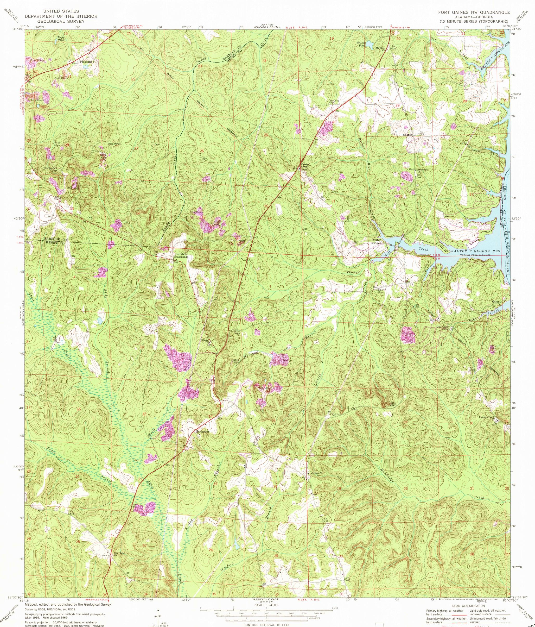
coordinate system, east zone. 1000-meter Universal Transverse Mercator grid ticks, zone 16, shown in blue. 1927 North American Datum. To place on the predicted North American Datum 1983 move the projection lines 15 meters south and 7 meters west as shown by dashed corner ticks
