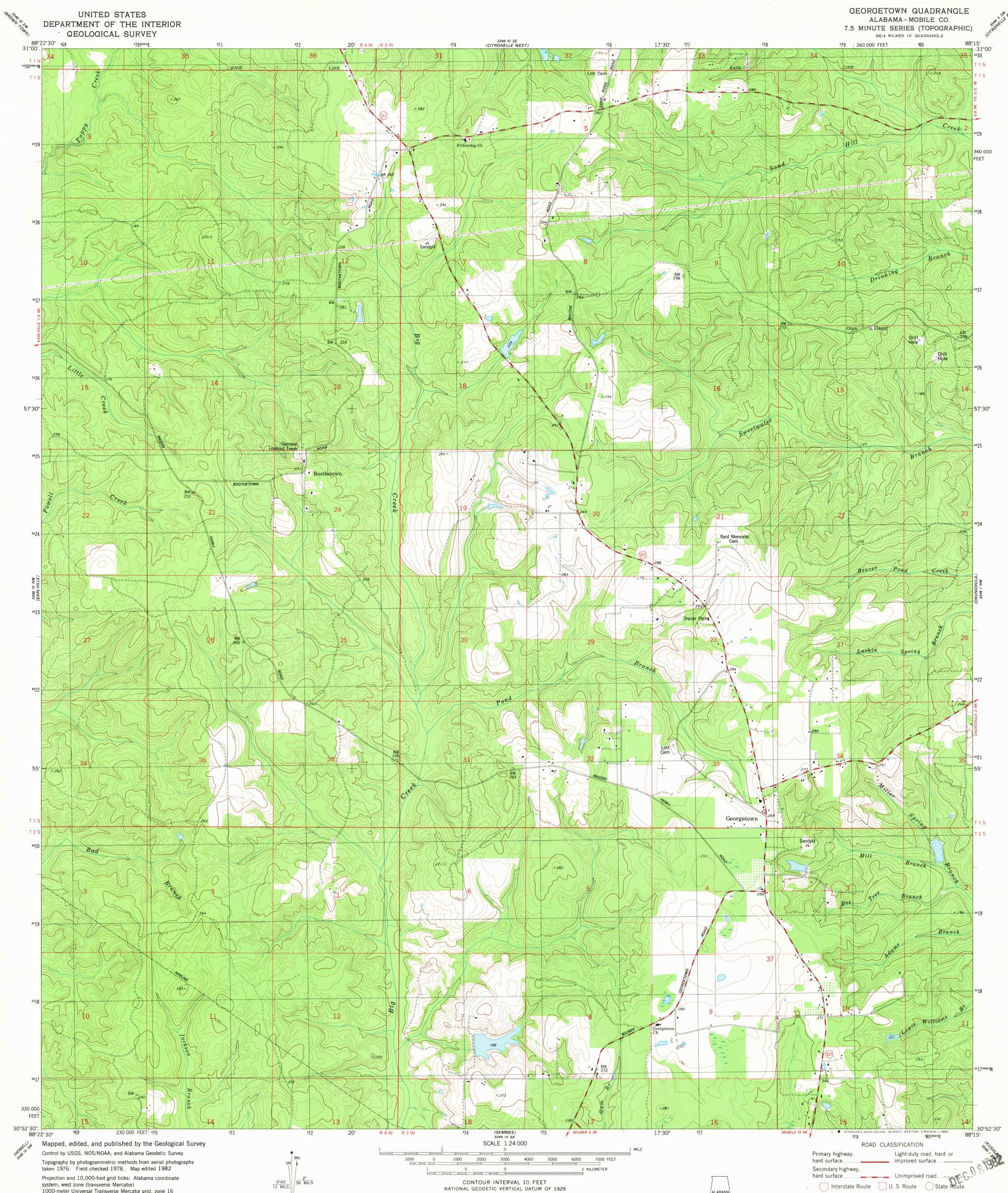
1000-meter Universal Transverse Mercator grid, zone 16 1927 North American Datum To place on the predicted North American Datum 1983 move the projection lines 16 meters south and 2 meters east as shown by dashed corner ticks
