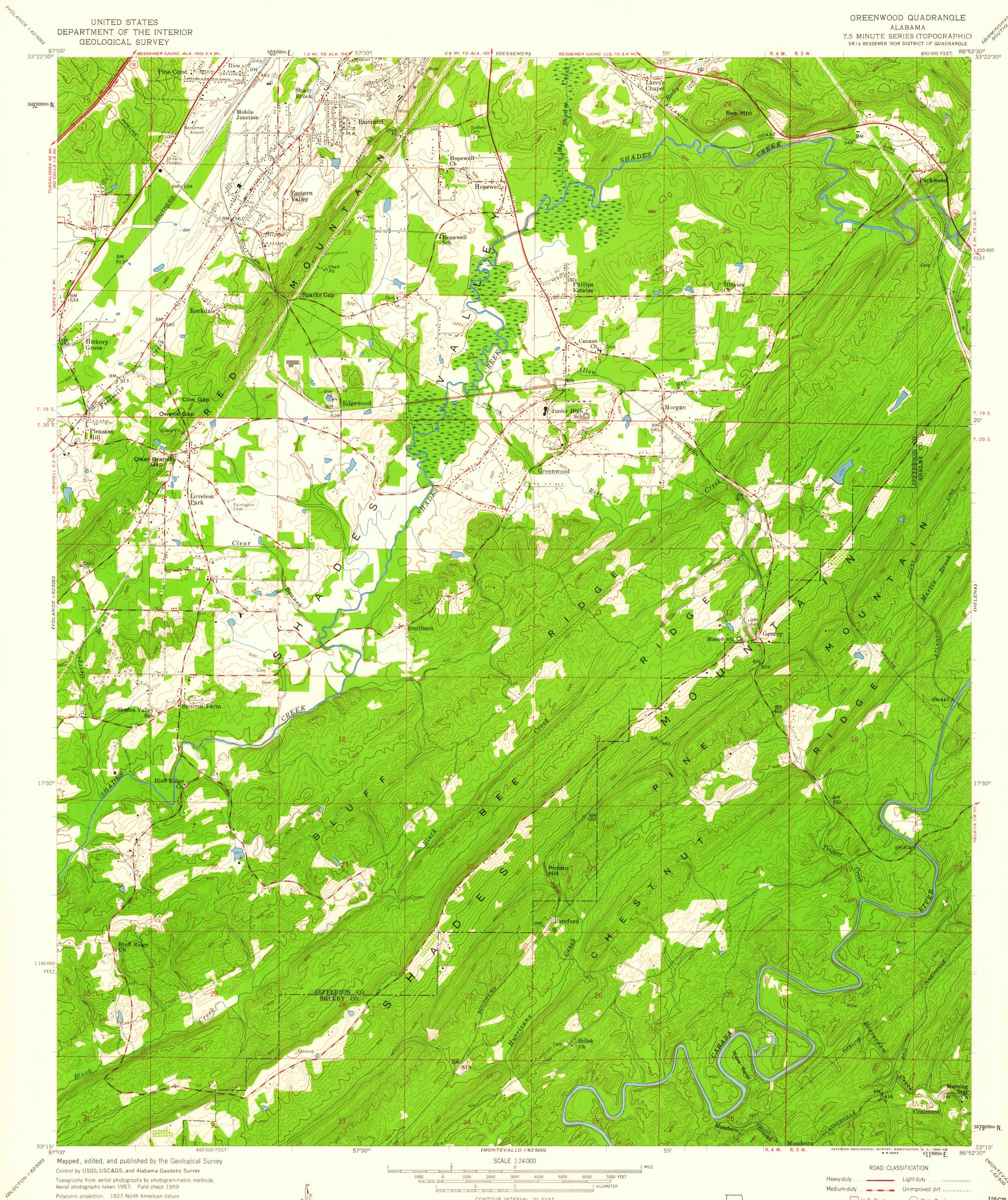
Aerial photographs taken 1957. Field check 1959 Polyconic projection. 1927 North American datum 10,000-foot grid based on Alabama coordinate system, west zone 1000-meter Universal Transverse Mercator grid ticks, zone 16, shown in blue
