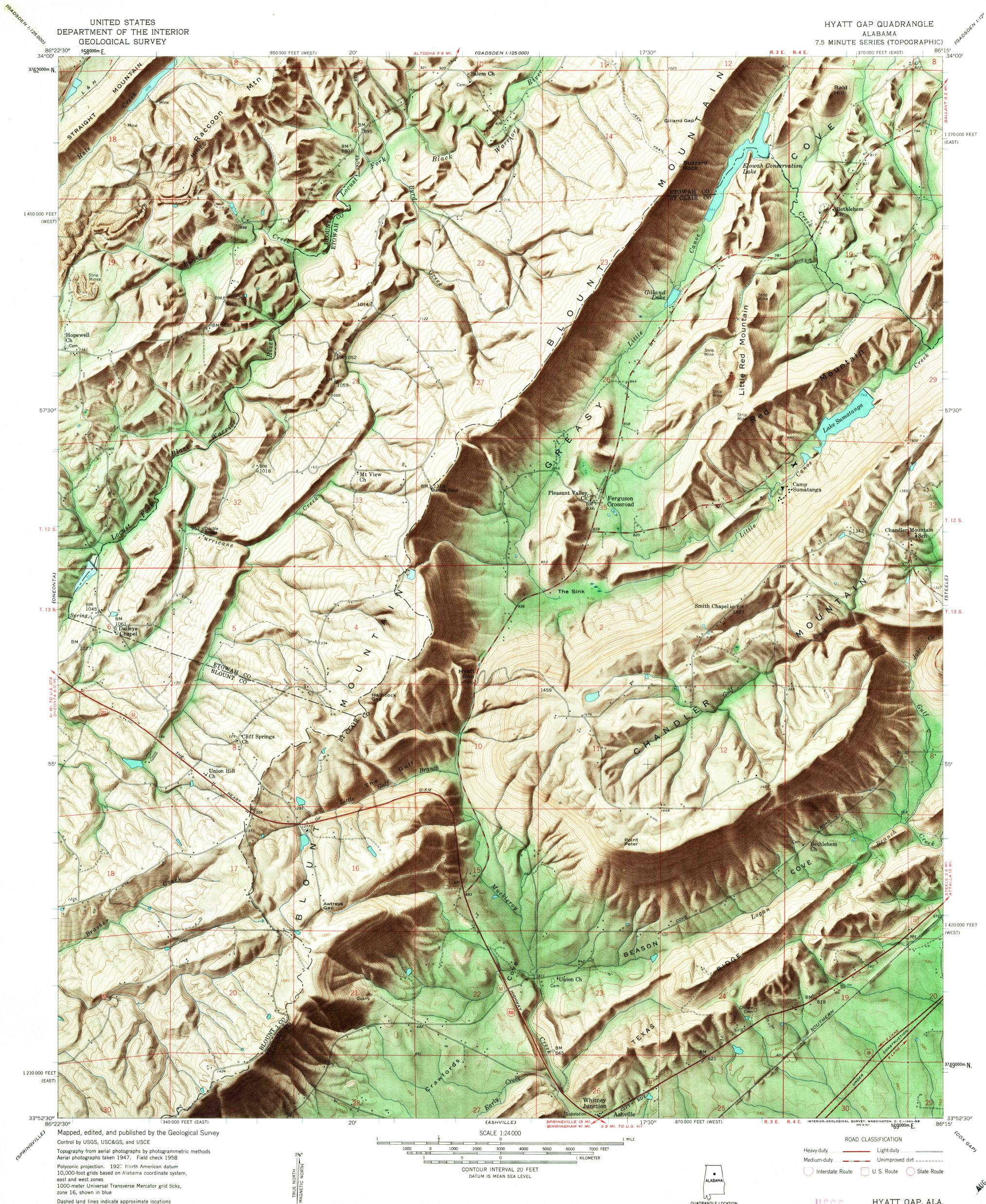
Polyconic projection. 1927 North American datum 10,000-foot grids based on Alabama coordinate system, east and west zones 1000-meter Universal Transverse Mercator grid ticks, zone 16, shown in blue
