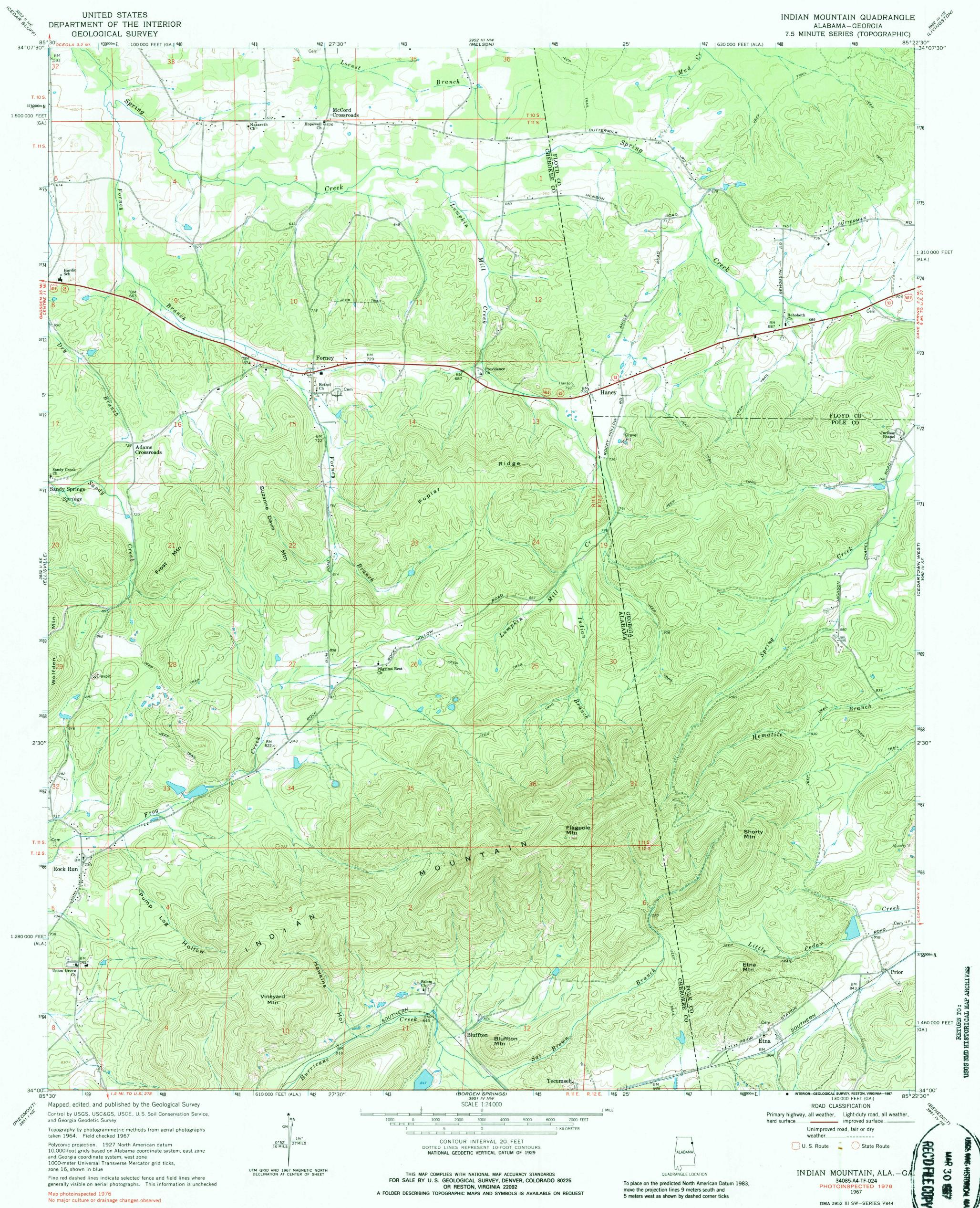
Polyconic projection. 1927 North American datum 10,000-foot grids based on Alabama coordinate system, east zone and Georgia coordinate system, west zone 1000-meter Universal Transverse Mercator grid ticks, zone 16, shown in blue
