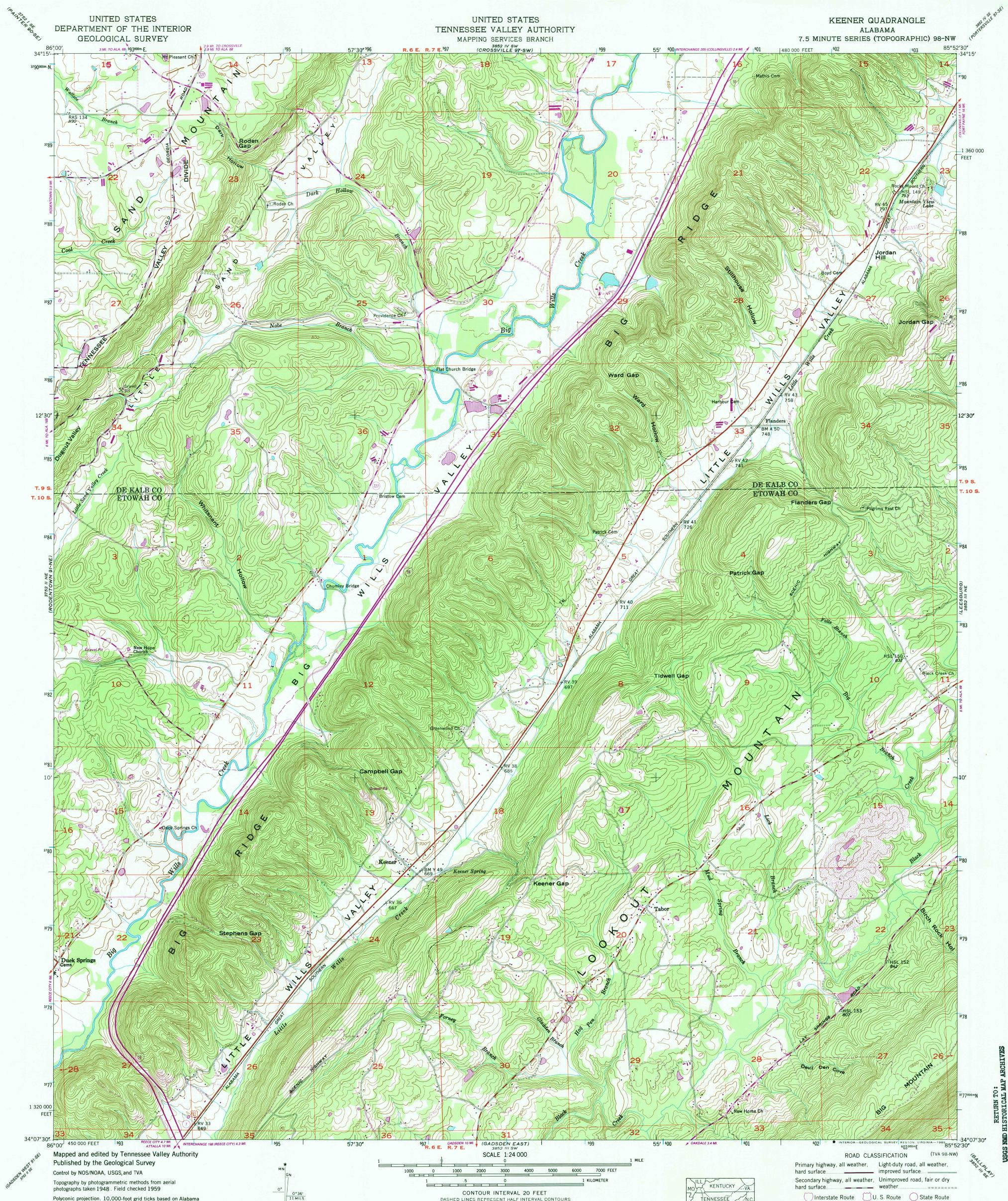
Polyconic projection. 10,000-foot grid ticks based on Alabama coordinate system, east zone. 1000-meter Universal Transverse Mercator grid ticks, zone 16, shown in blue 1927 North American Datum To place on the predicted North American Datum 1983 move the projection lines 9 meters south and 3 meters west as shown by dashed corner ticks Fine red dashed lines indicate selected fence and field lines
