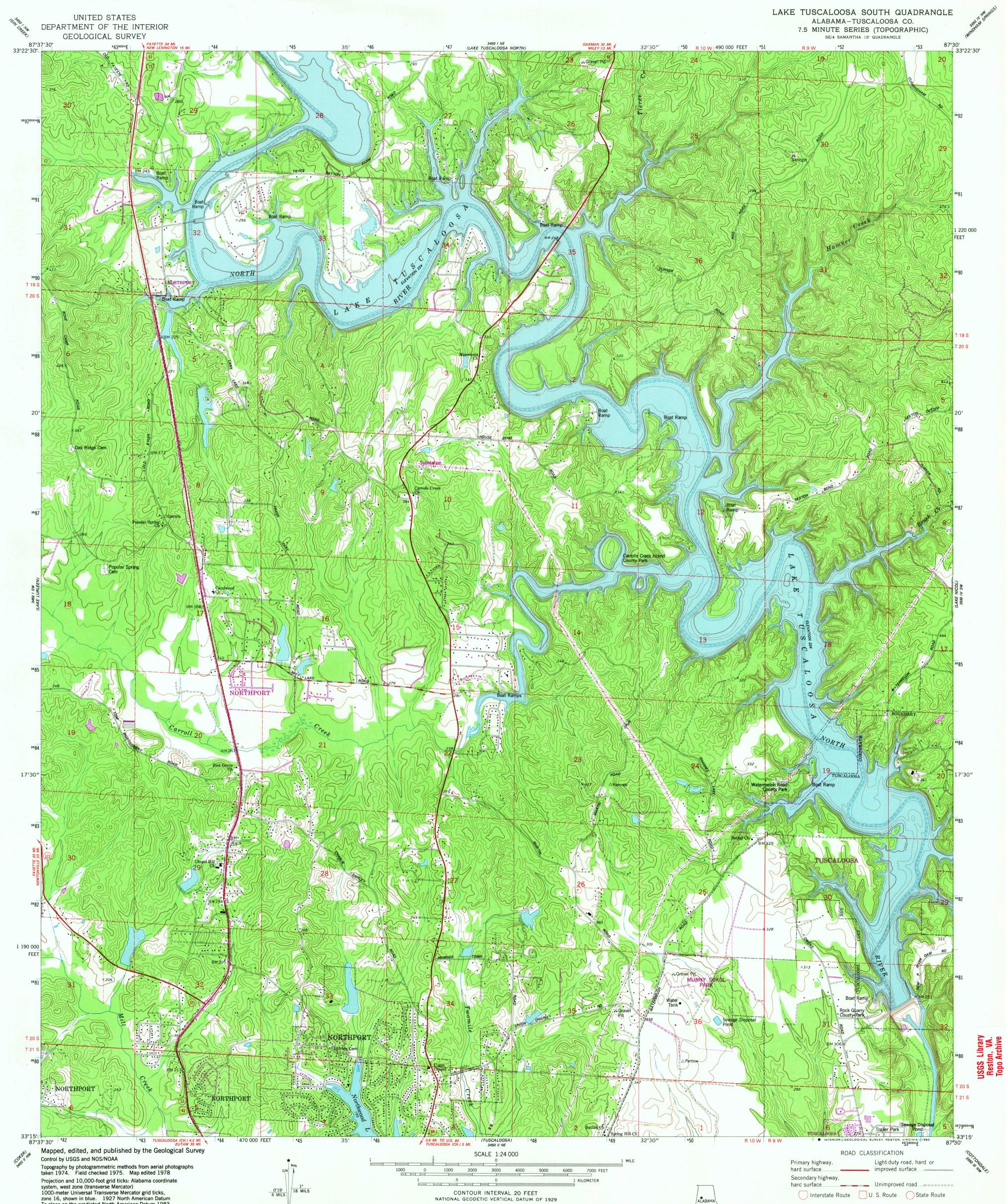
1000-meter Universal Transverse Mercator grid ticks, zone 16, shown in blue. 1927 North American Datum To place on the predicted North American Datum 1983 move the projection lines 10 meters south and 1 meter east as shown by dashed corner ticks
