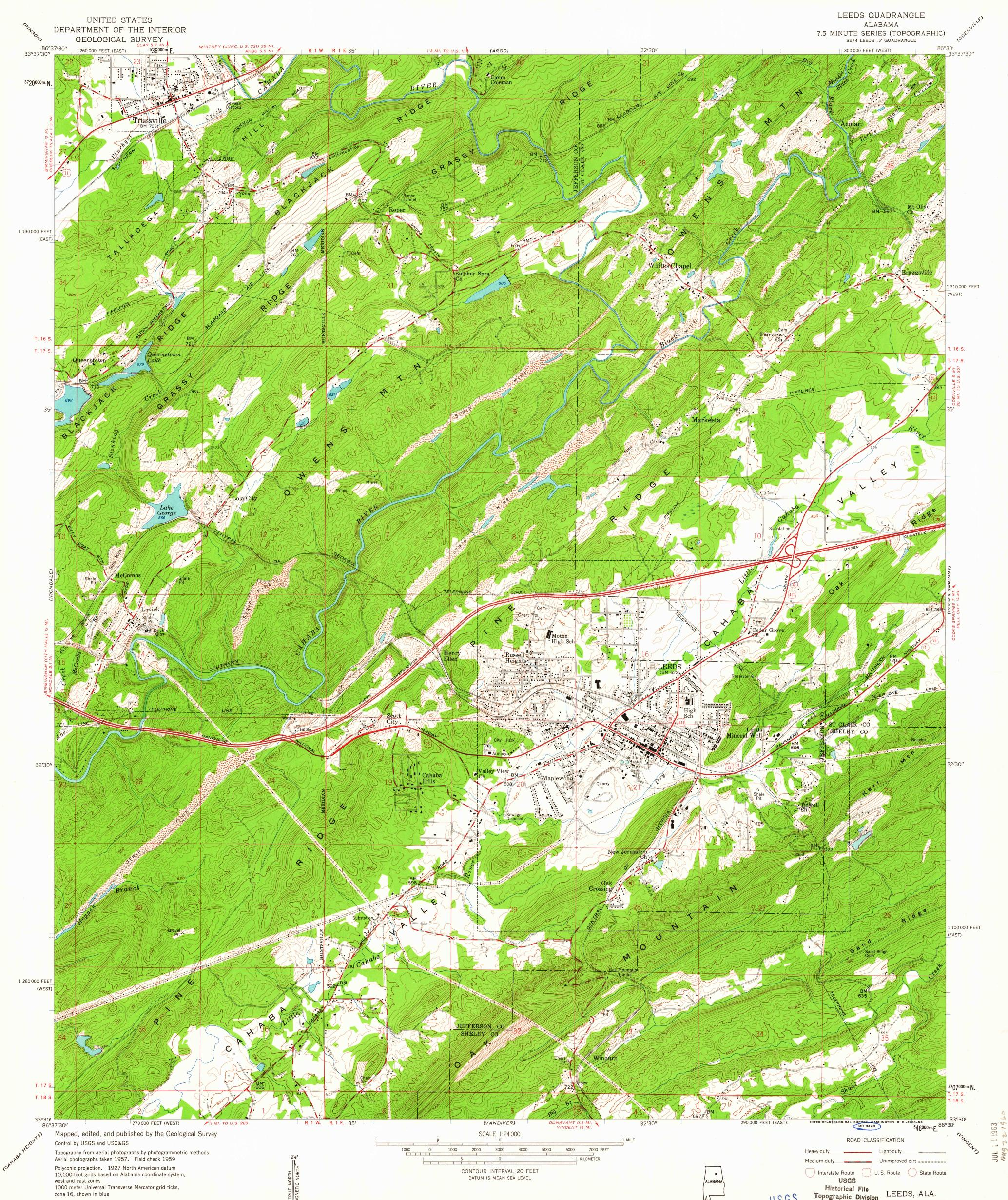
Polyconic projection. 1927 North American datum 10,000-foot grids based on Alabama coordinate system, west and east zones 1000-meter Universal Transverse Mercator grid ticks, zone 16, shown in blue
