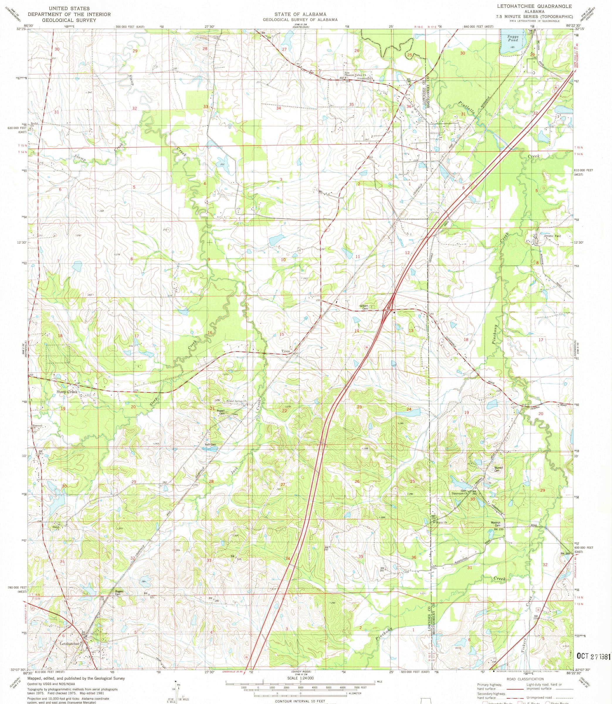
system, west and east zones (transverse Mercator) 1000-meter Universal Transverse Mercator grid, zone 16 1927 North American Datum To place on the predicted North American Datum 1983 move the projection lines 13 meters south and 3 meters west as shown by dashed corner ticks
