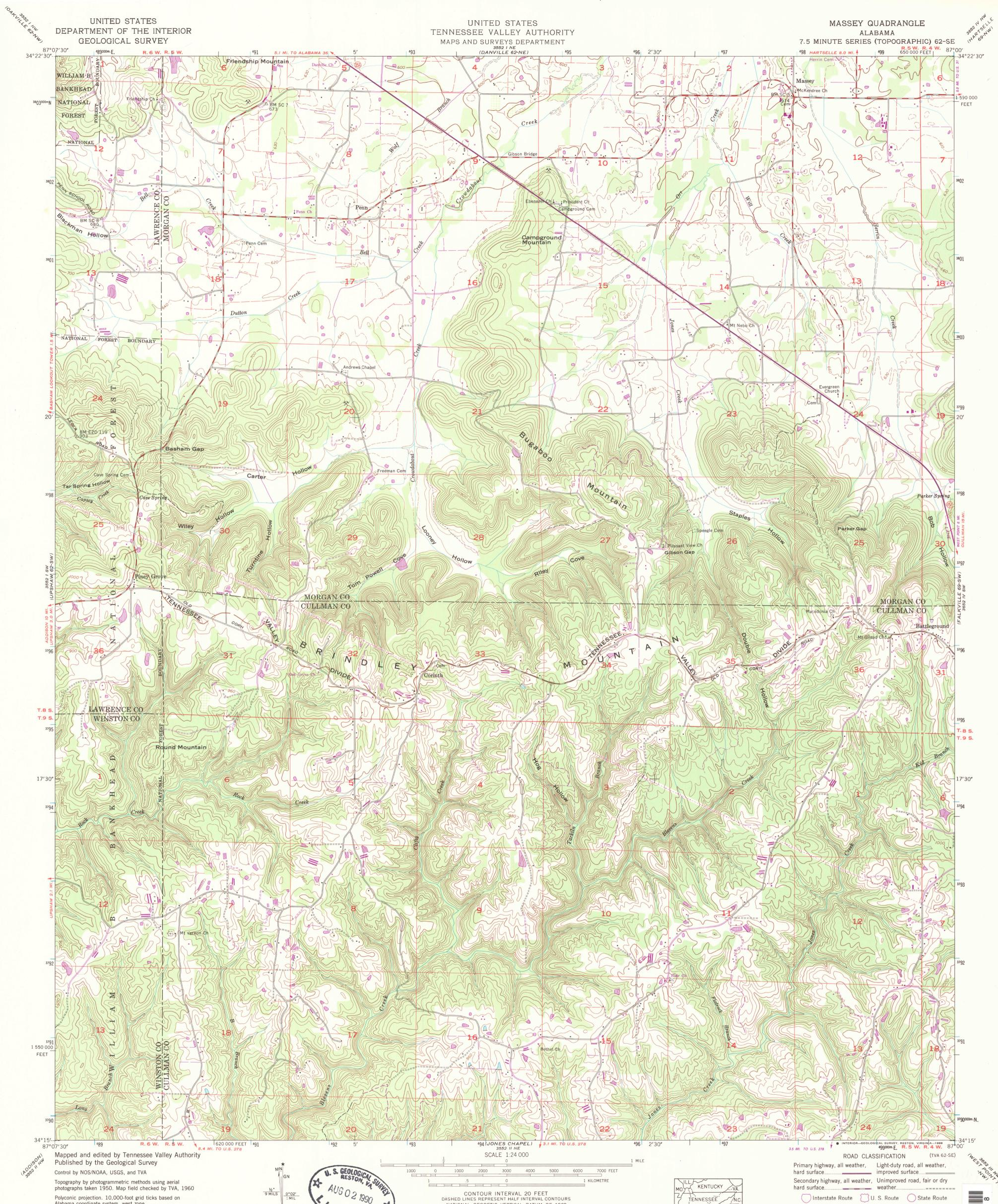
Polyconic projection. 10,000-foot grid ticks based on Alabama coordinate system, west zone 1000-meter Universal Transverse Mercator grid ticks, zone 16, shown in blue. 1927 North American Datum To place on the predicted North American Datum 1983 move the projection lines 8 meters south as shown by dashed corner ticks
