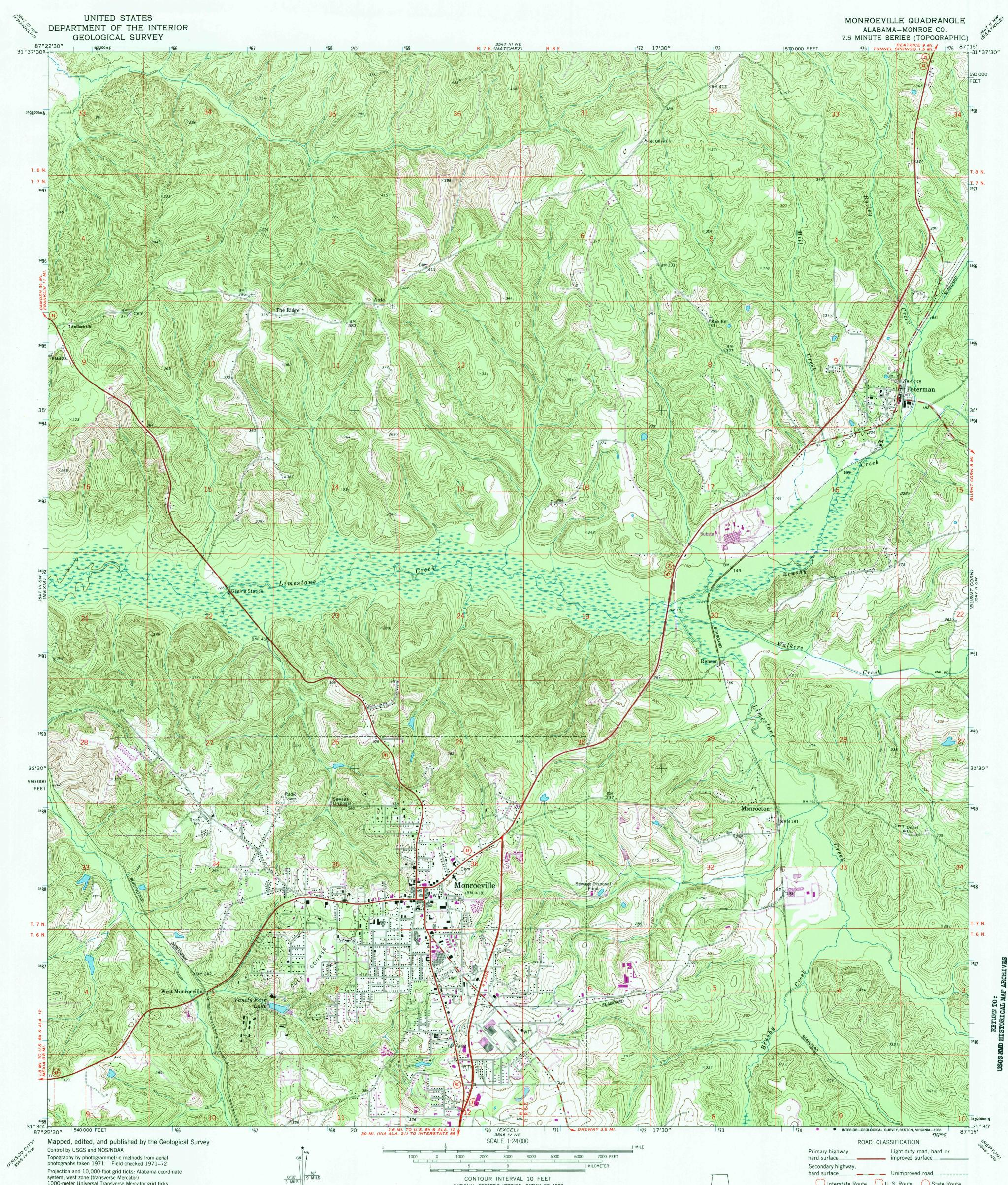
1000-meter Universal Transverse Mercator grid ticks, zone 16, shown in blue 1927 North American Datum To place on the predicted North American Datum 1983 move the projection lines 14 meters south and 1 meter west as shown by dashed corner ticks
