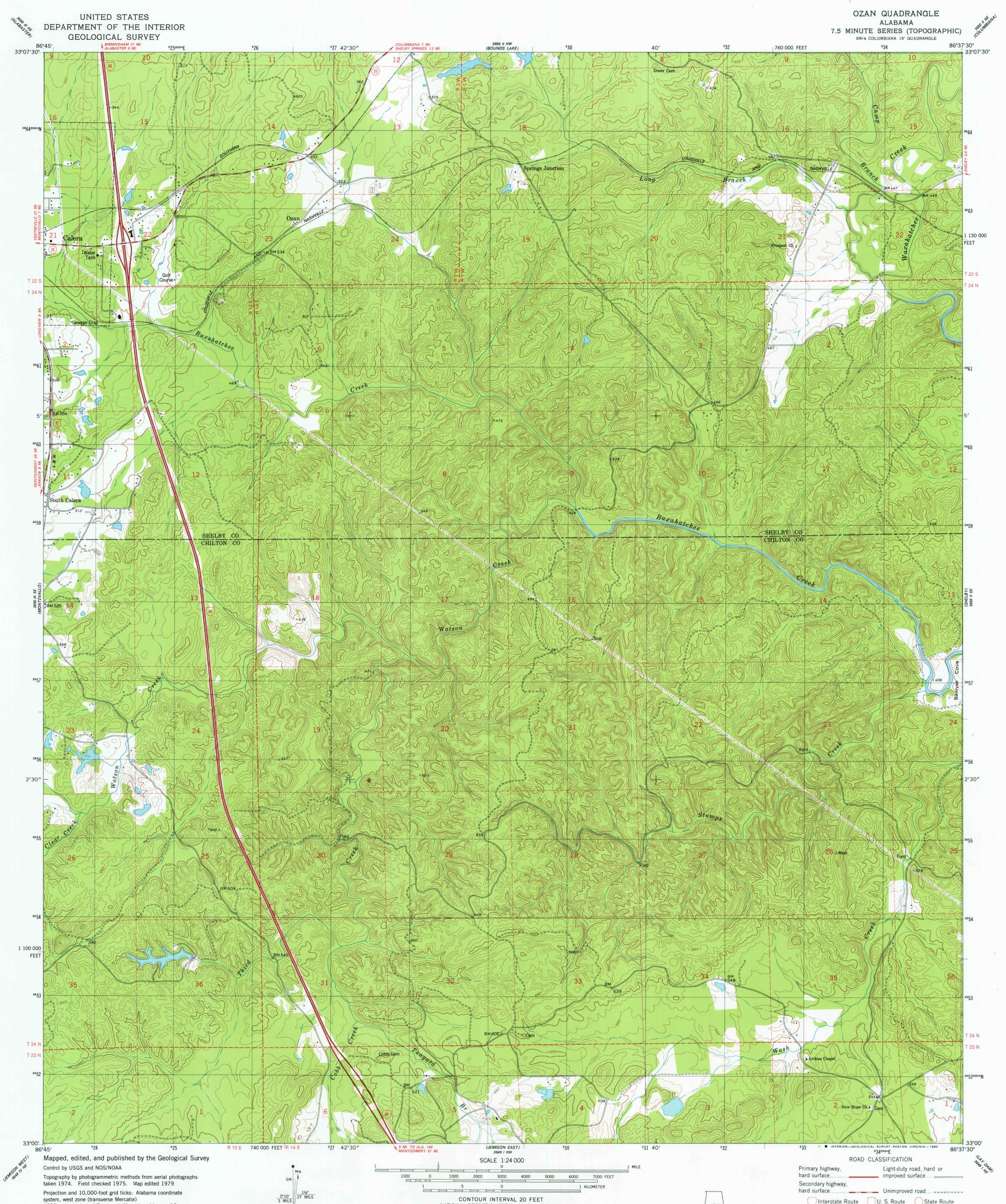
system, west zone (transverse Mercator) 1000-meter Universal Transverse Mercator grid, zone 16 1927 North American Datum To place on the predicted North American Datum 1983 move the projection lines 10 meters south and 2 meters west as shown by dashed corner ticks
