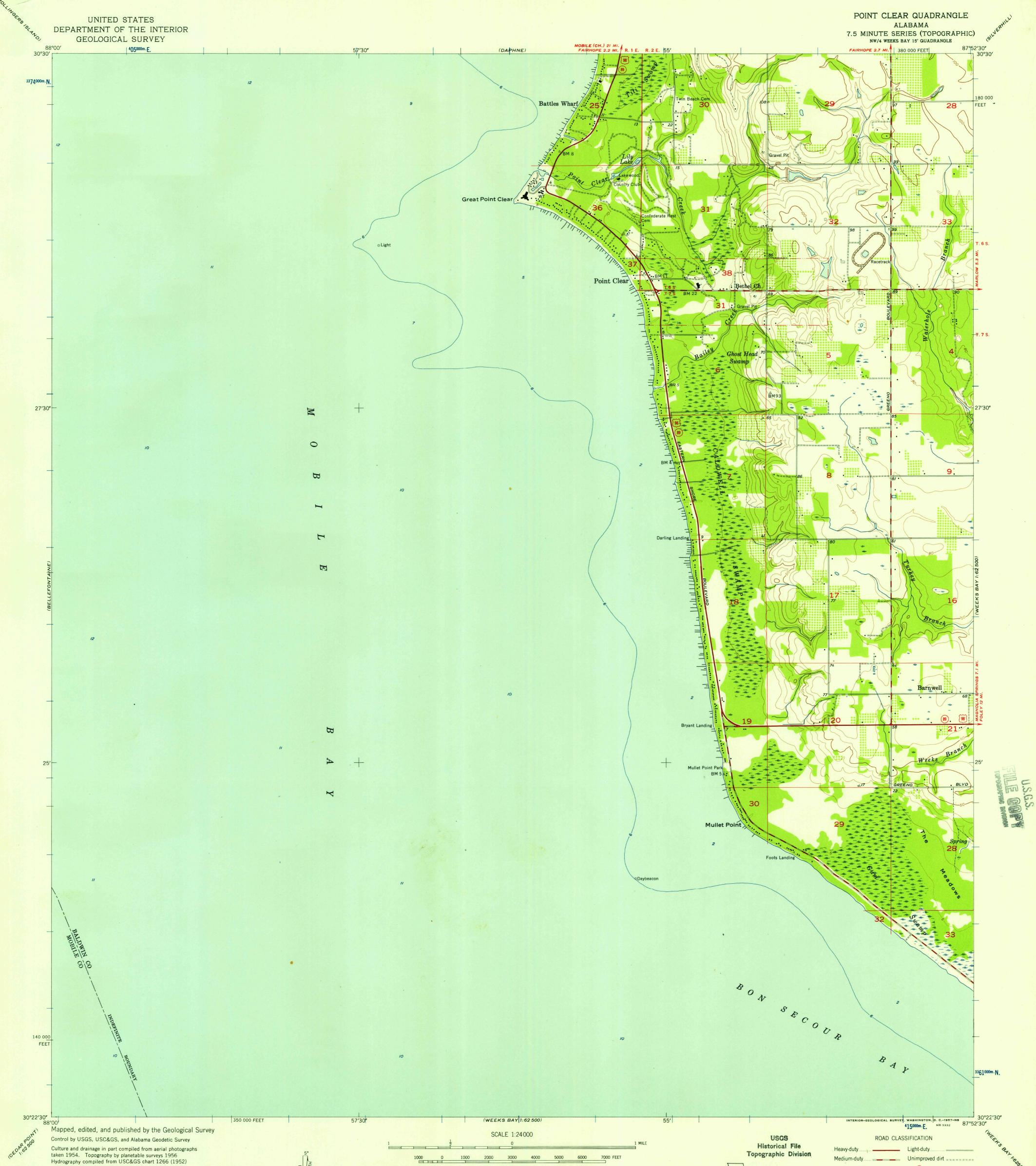
Polyconic projection. 1927 North American datum 10,000-foot grid based on Alabama coordinate system, west zone 1000-meter Universal Transverse Mercator grid ticks, zone 16, shown in blue
