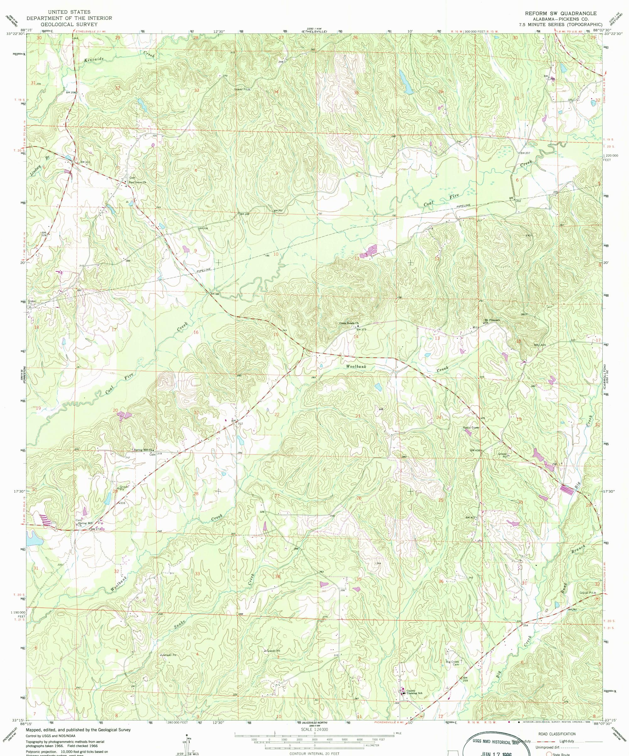
Alabama coordinate system, west zone 1000-meter Universal Transverse Mercator grid ticks, zone 16, shown in blue 1927 North American Datum To place on the predicted North American Datum 1983 move the projection lines 11 meters south and 2 meters east as shown by dashed corner ticks Fine red dashed lines indicate selected fence and field lines where generally visible on aerial photographs. This information is unchecked
