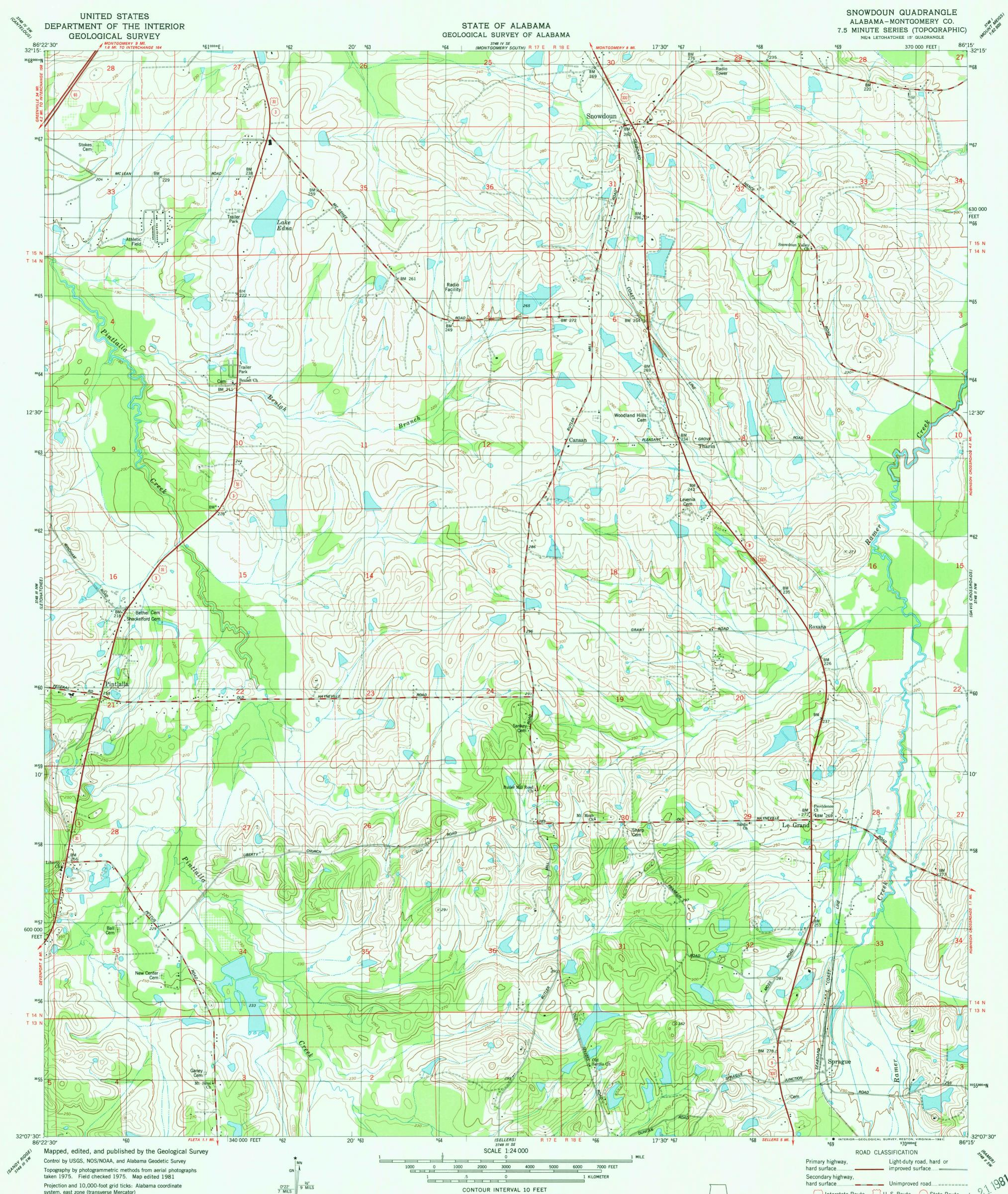
system, east zone (transverse Mercator) 1000-meter Universal Transverse Mercator grid, zone 16 1927 North American Datum To place on the predicted North American Datum 1983 move the projection lines 13 meters south and 3 meters west as shown by dashed corner ticks
