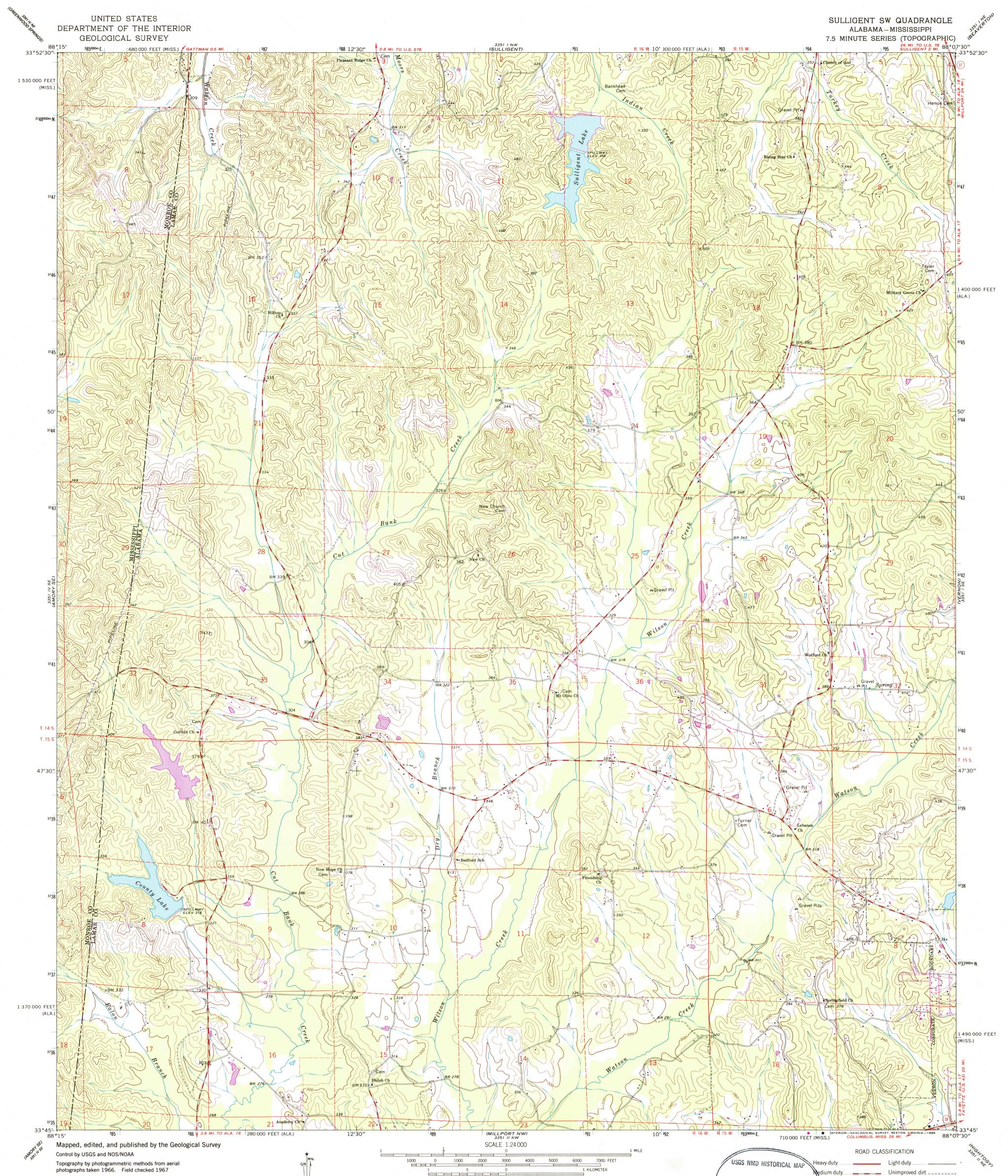
Polyconic projection. 10,000-foot grid ticks based on Alabama coordinate system, west zone, and Mississippi coordinate system, east zone 1000-meter Universal Transverse Mercator grid ticks, zone 16, shown in blue 1927 North American Datum To place on the predicted North American Datum 1983 move the projection lines 10 meters south and 3 meters east as shown by dashed corner ticks
