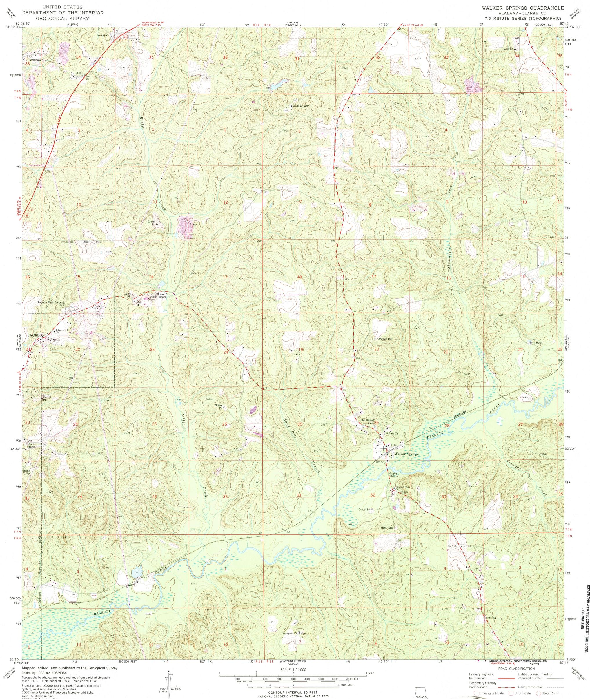
Projection and 10,000-foot grid ticks: Alabama coordinate system, west zone (transverse Mercator) 1000-meter Universal Transverse Mercator grid ticks, zone 16, shown in blue 1927 North American Datum To place on the predicted North American Datum 1983 move the projection lines 15 meters south as shown by dashed corner ticks as shown by dashed corner ticks
