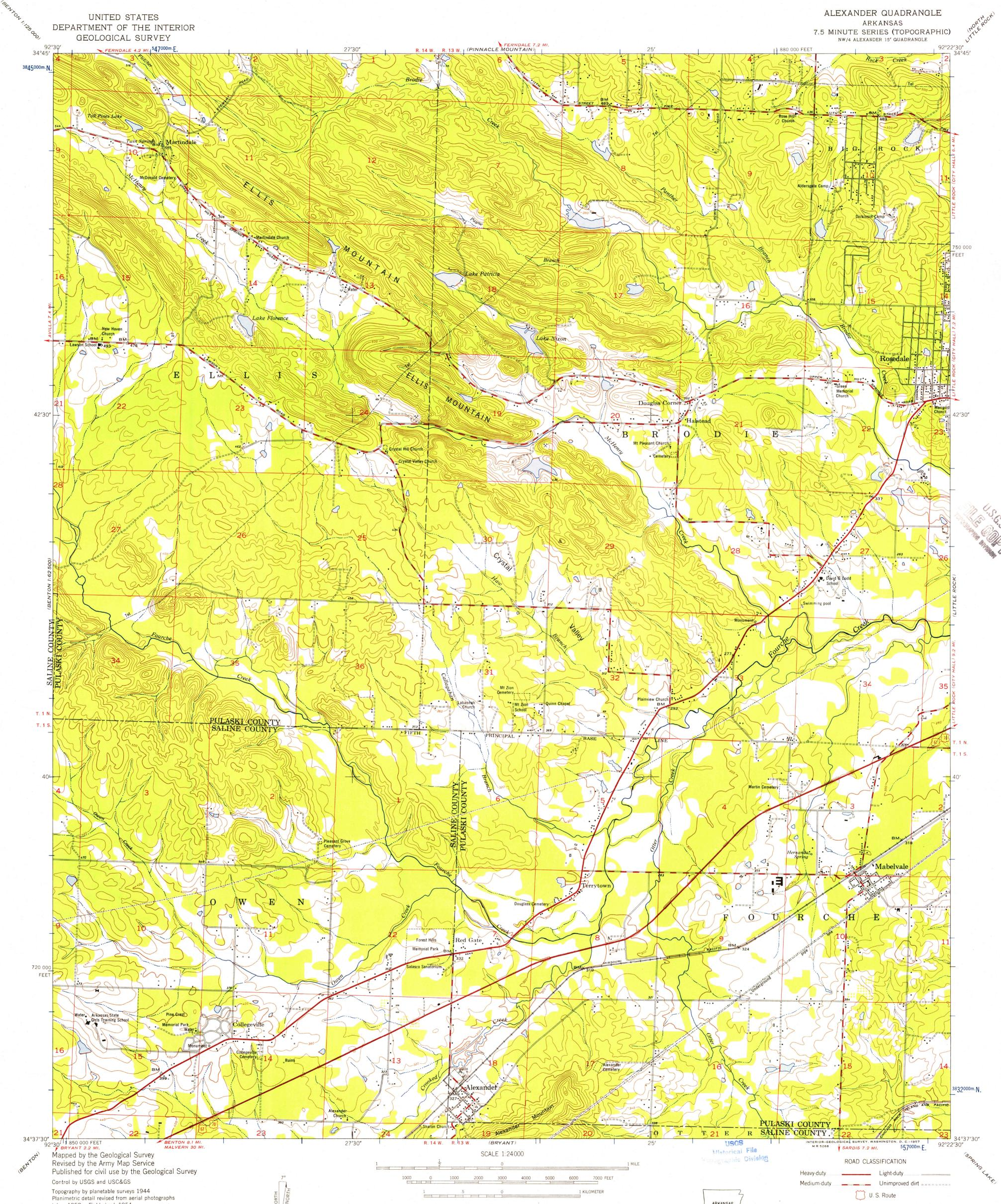
Topography by planetable surveys 1944 Planimetric detail revised from aerial photographs taken 1952. Field check 1954
