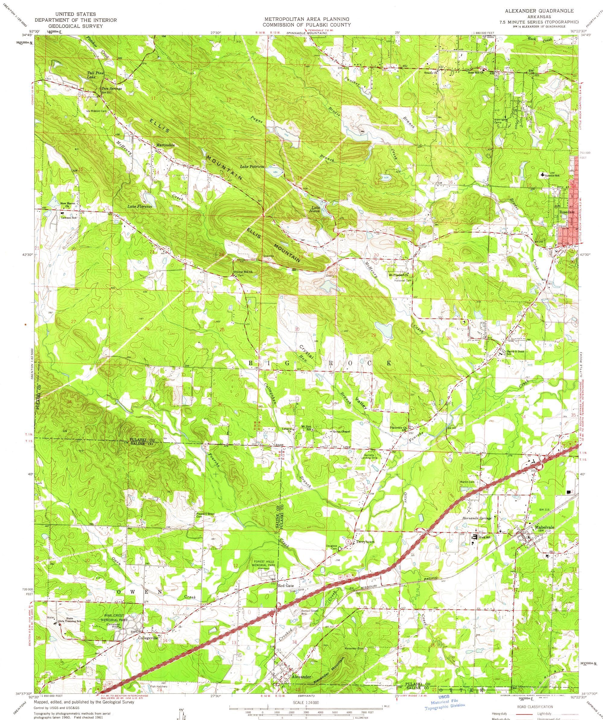
Polyconic projection. 1927 North American datum 10,000-foot grid based on Arkansas coordinate system, south zone 1000-meter Universal Transverse Mercator grid ticks, zone 15, shown in blue Red tint indicates area in which only landmark buildings are shown Fine red dashed lines indicate selected fence and field lines where generally visible on aerial photographs. This information is unchecked APPROXIMATE MEAN DECLINATION, 1961
