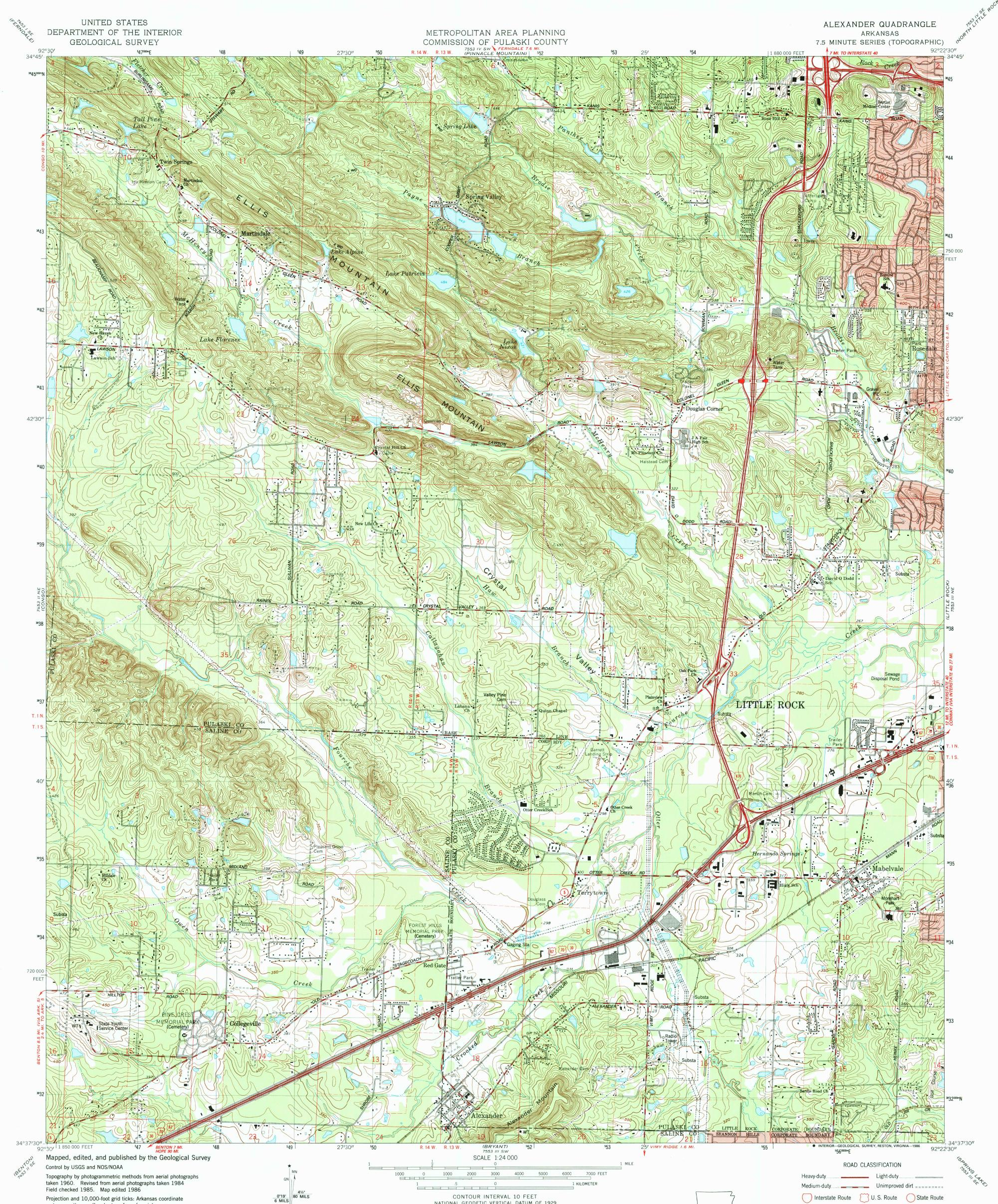
Projection and 10,000-foot grid ticks: Arkansas coordinate system, south zone (Lambert conformal conic) 1000-meter Universal Transverse Mercator grid, zone 15 1927 North American Datum To place on the predicted North American Datum 1983, move the projection lines 8 meters south and 14 meters east as shown by dashed corner ticks Red tint indicates areas in which only landmark buildings are shown Fine red dashed lines indicate selected fence and field lines where
