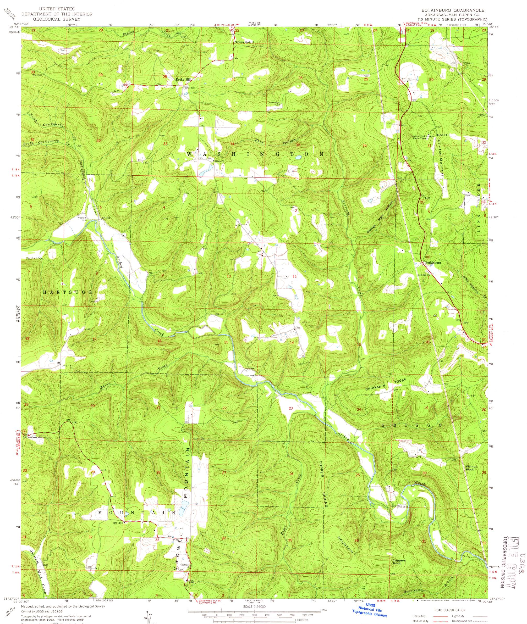
Polyconic projection. 1927 North American datum 10,000-foot grid based on Arkansas coordinate system, north zone 1000-meter Universal Transverse Mercator grid ticks, zone 15, shown in blue
