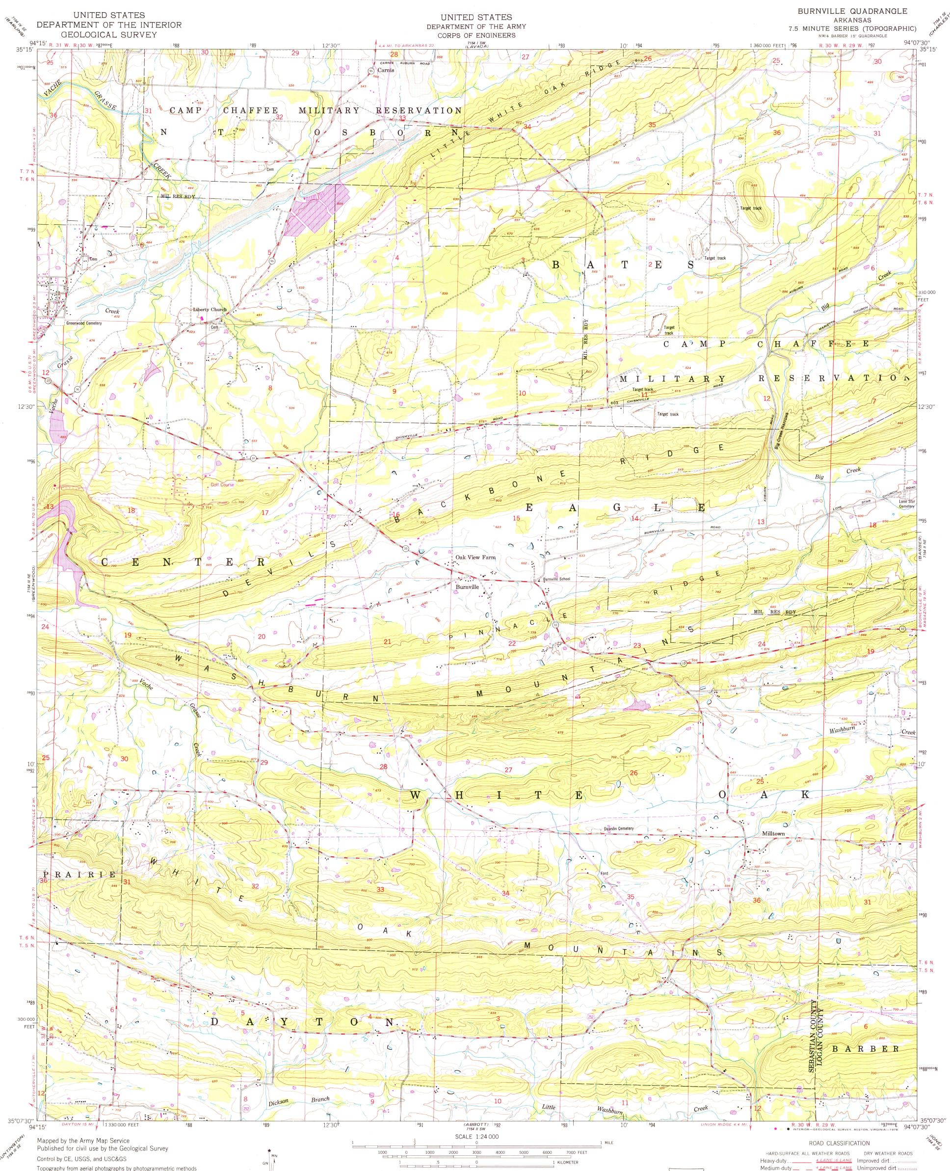
Aerial photographs taken 1946. Field check 1947 Polyconic projection. 1927 North American datum 10,000-foot grid based on Arkansas coordinate system, north zone
