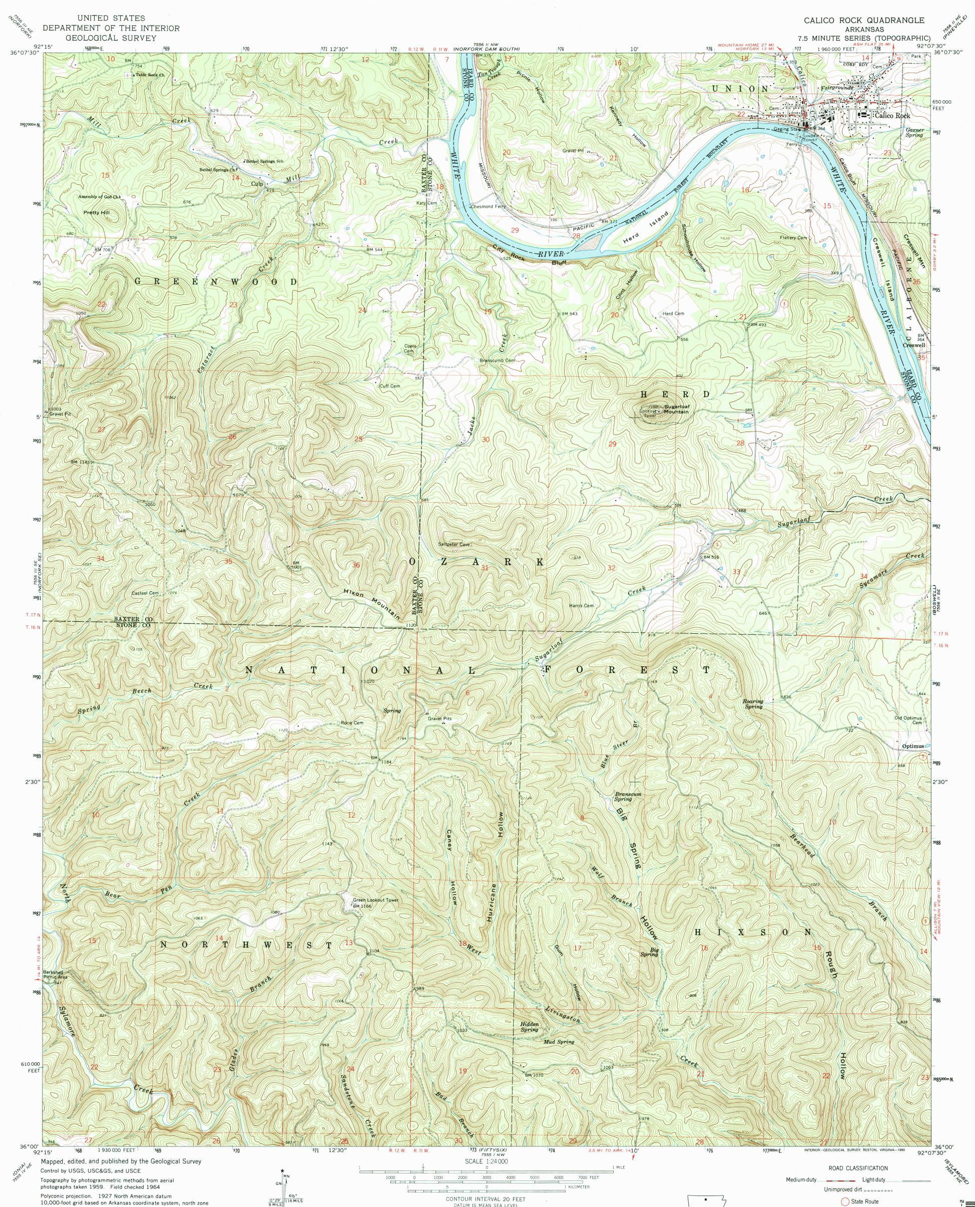
10,000-foot grid based on Arkansas coordinate system, north zone 1000-meter Universal Transverse Mercator grid ticks, zone 15, shown in blue
