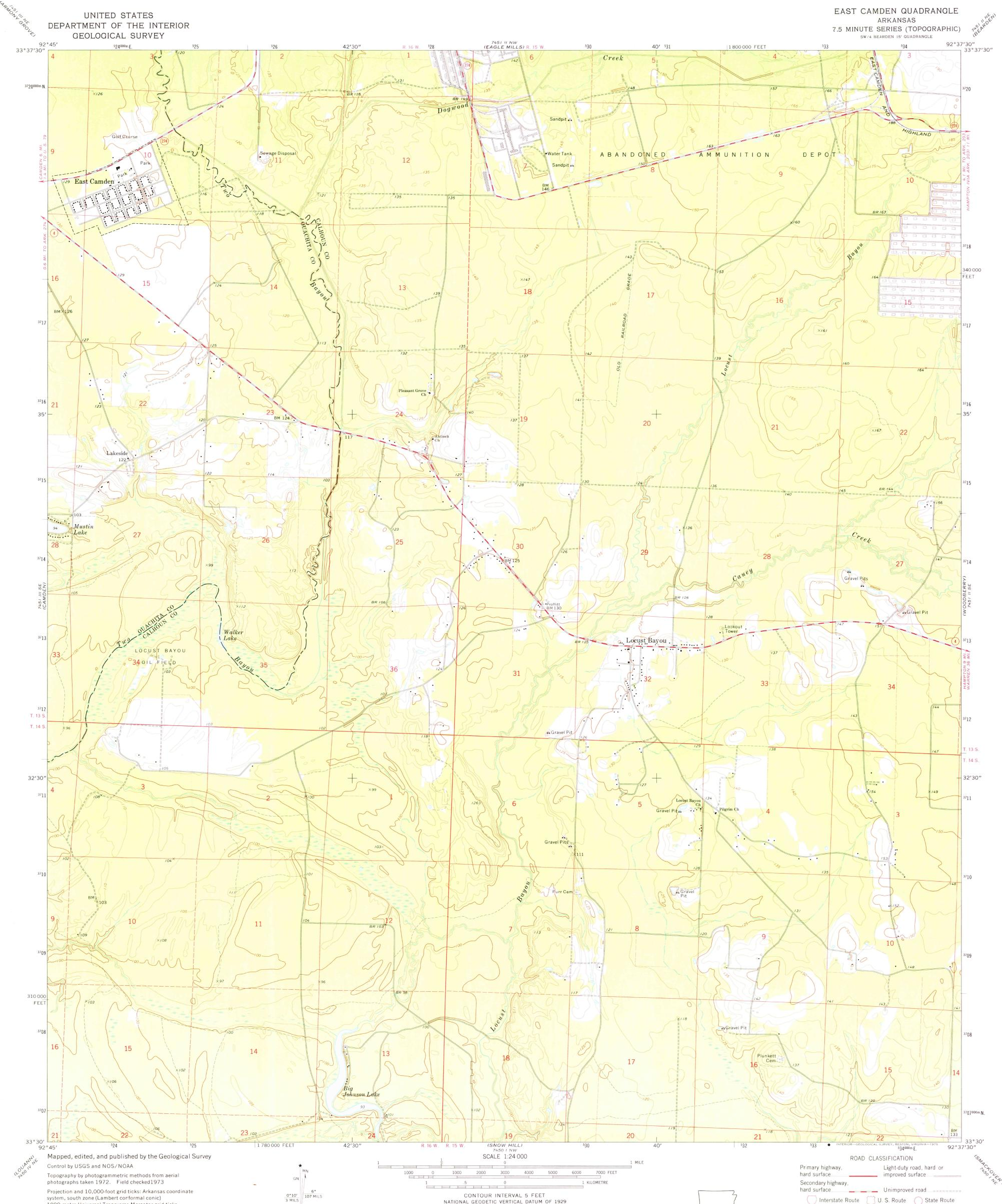
Projection and 10,000-foot grid ticks: Arkansas coordinate system, south zone (Lambert conformal conic) 1000-metre Universal Transverse Mercator grid ticks, zone 15, shown in blue. 1927 North American datum
