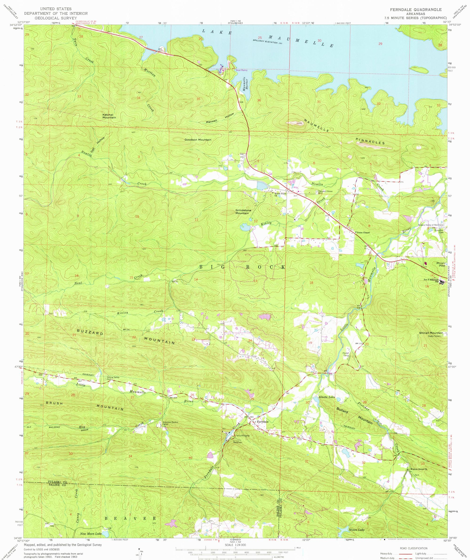
Polyconic projection. 1927 North American datum 10,000-foot grid based on Arkansas coordinate system, south zone 1000-metre Universal Transverse Mercator grid ticks, zone 15, shown in blue
