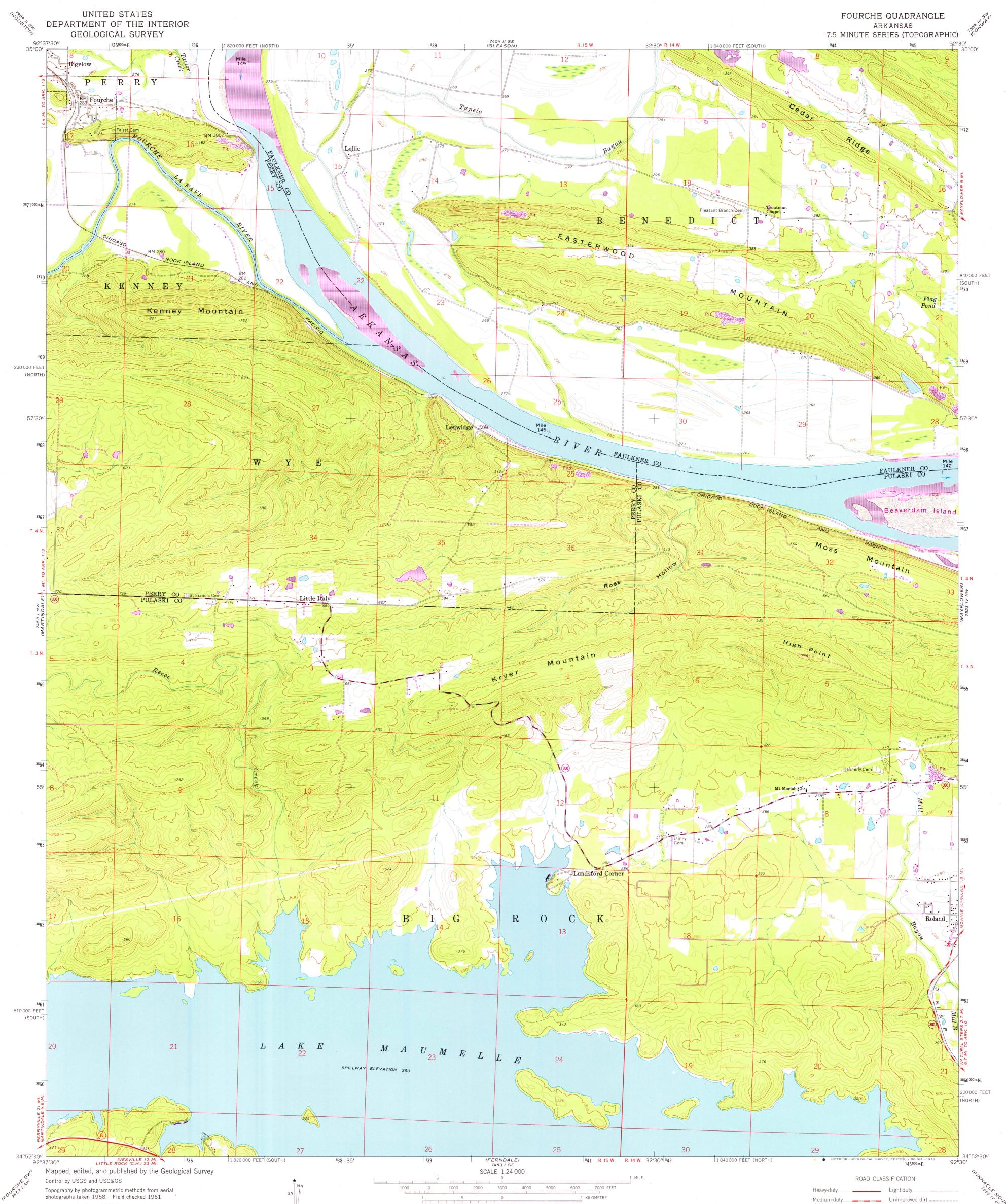
Polyconic projection. 1927 North American datum 10,000-foot grids based on Arkansas coordinate system, north and south zones 1000-metre Universal Transverse Mercator grid ticks, zone 15, shown in blue
