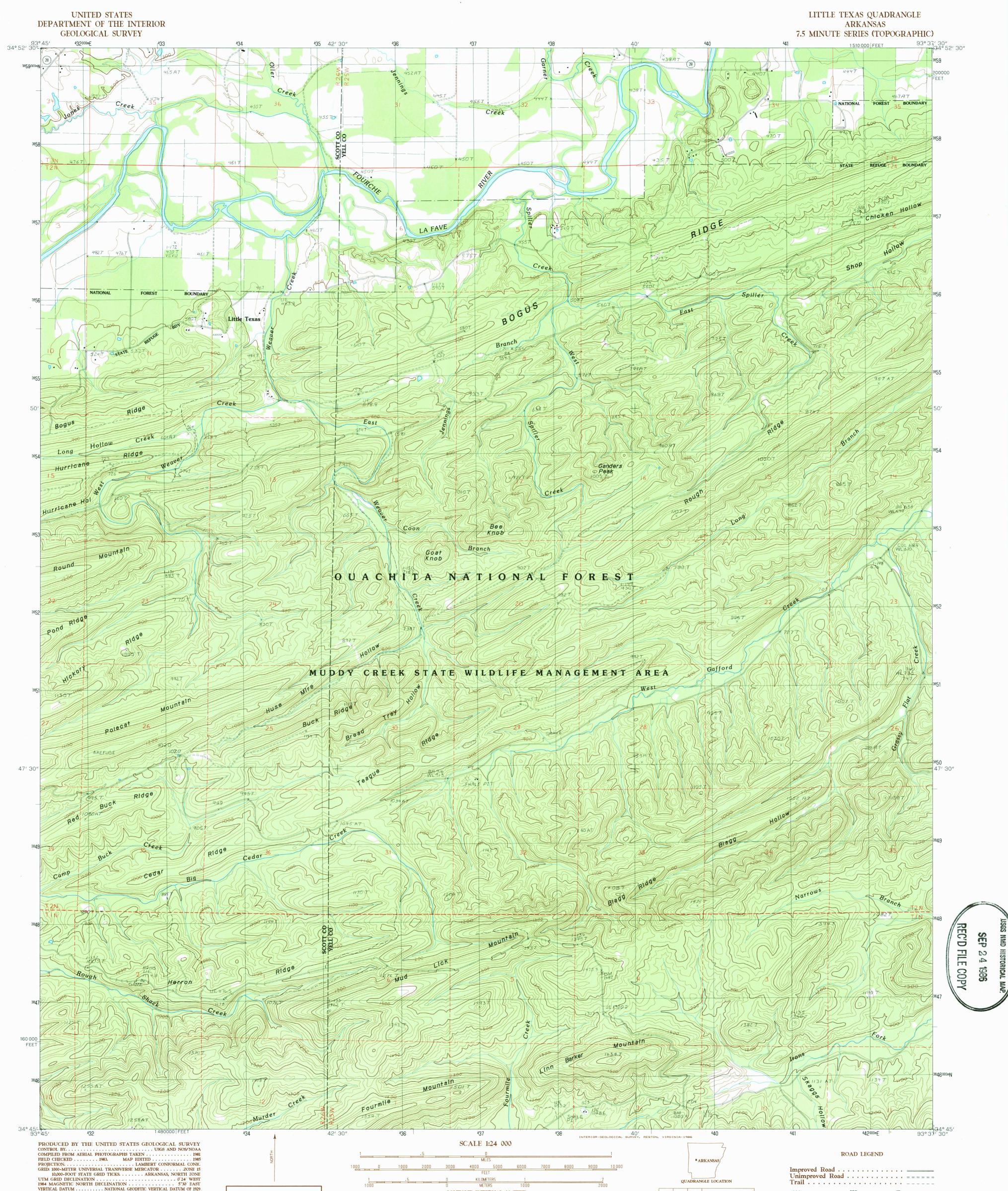
VERTICAL DATUM ...... NATIONAL GEODETIC VERTICAL DATUM OF 1929 HORIZONTAL DATUM ...... 1927 NORTH AMERICAN DATUM To place on the predicted North American Datum of 1983, move the projection lines as shown by dashed corner ticks (7 meters south and 17 meters east) There may be private inholdings within the boundaries of any Federal and State Reservations shown on this map No distinction made between houses, barns, and other buildings
