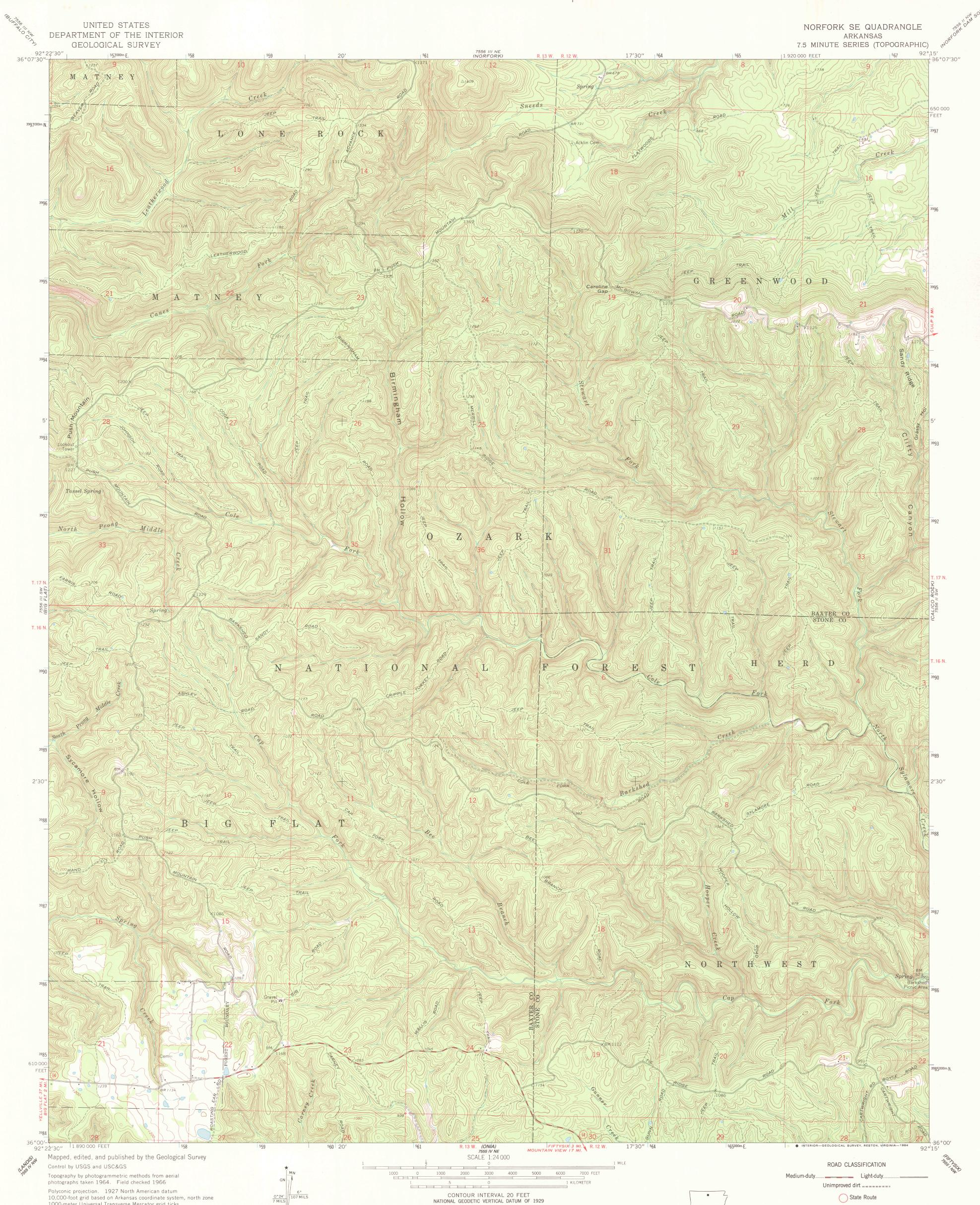
Polyconic projection. 1927 North American datum 10,000-foot grid based on Arkansas coordinate system, north zone 1000-meter Universal Transverse Mercator grid ticks, zone 15, shown in blue To place on the predicted North American Datum 1983, move the projection lines 5 meters south and 14 meters east as shown by dashed corner ticks There may be private inholdings within the boundaries of the National or State reservations shown on this map
