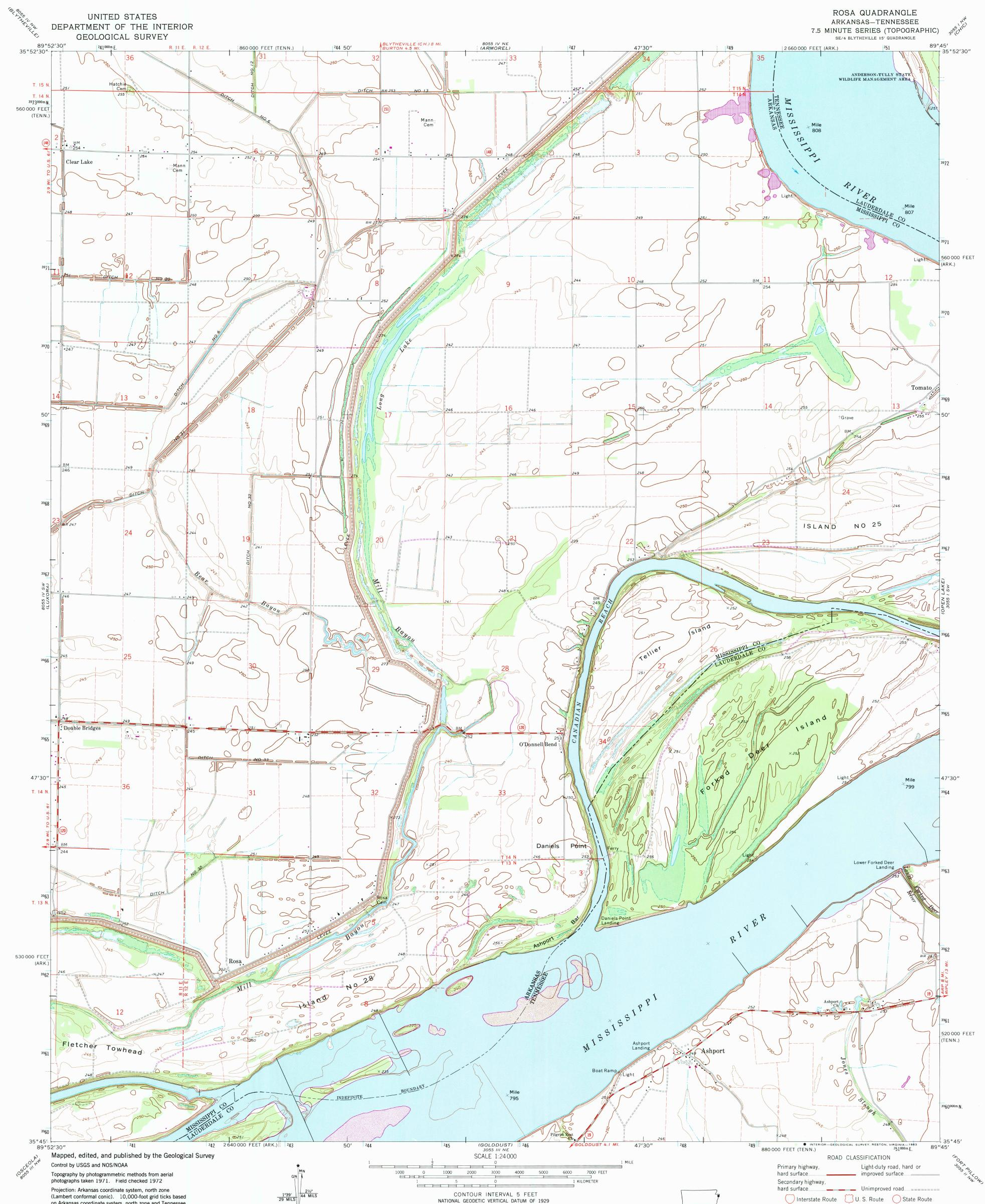
(Lambert conformal conic). 10,000-foot grid ticks based on Arkansas coordinate system, north zone and Tennessee coordinate system. 1000-meter Universal Transverse Mercator grid ticks, zone 16, shown in blue. 1927 North American Datum To place on the predicted North American Datum 1983 move the projection lines 6 meters south and 8 meters east as shown by dashed corner ticks
