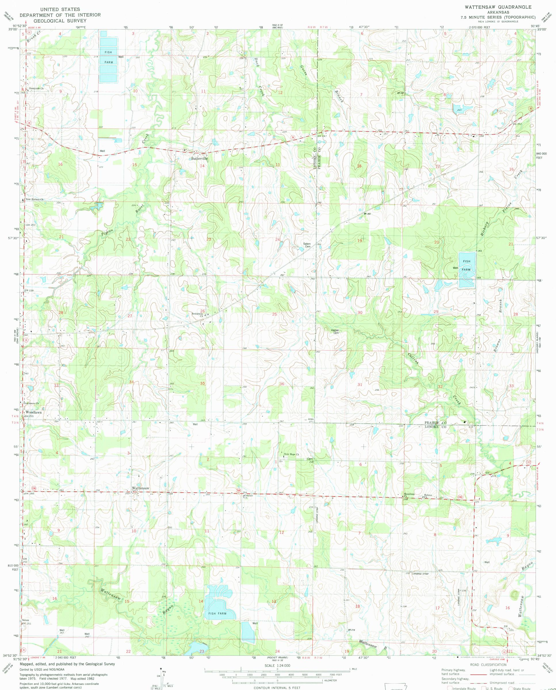
1000-meter Universal Transverse Mercator grid, zone 15 1927 North American Datum To place on the predicted North American Datum 1983 move the projection lines 7 meters south and 13 meters east as shown by dashed corner ticks
