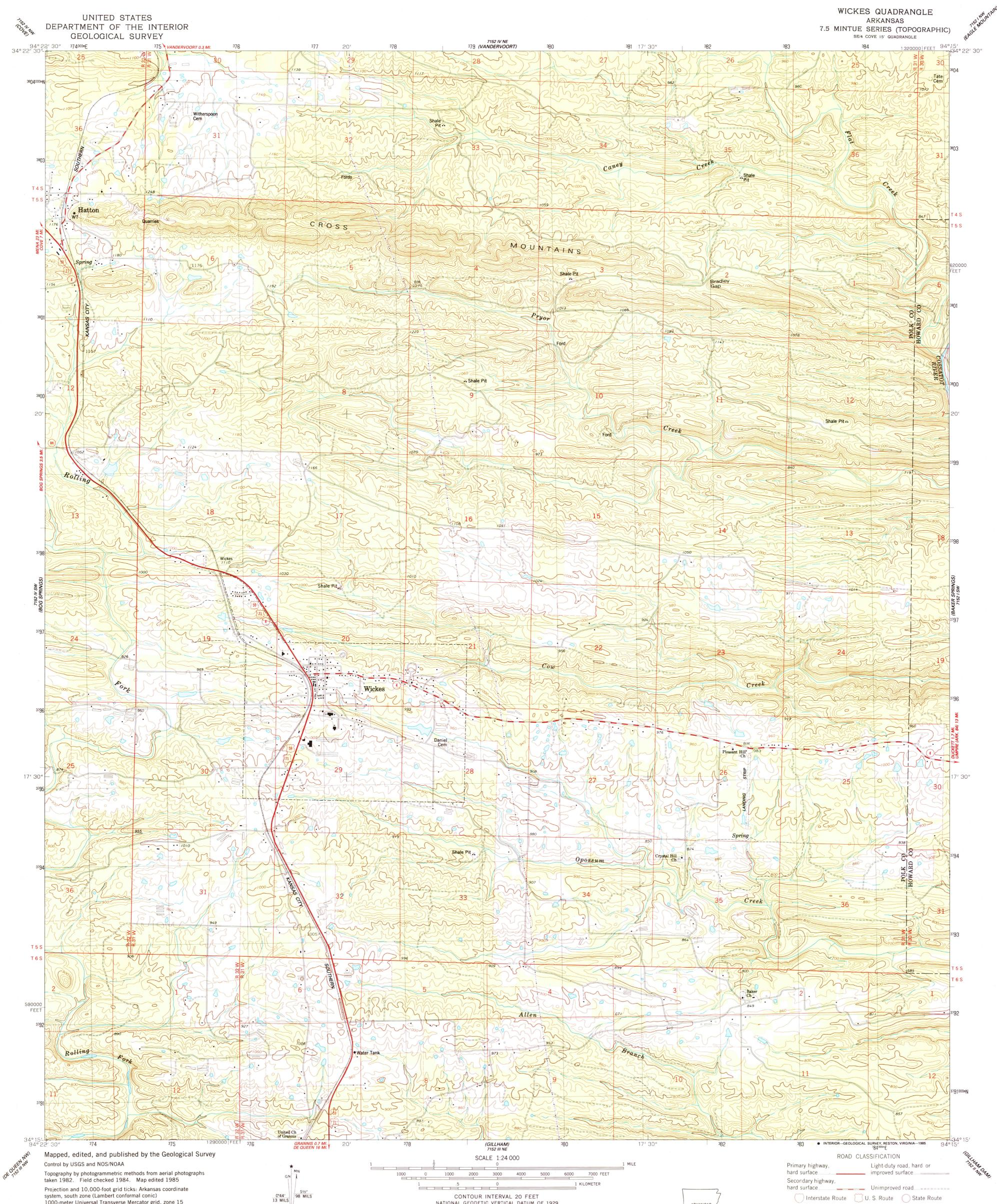
system, south zone (Lambert conformal conic) 1000-meter Universal Transverse Mercator grid, zone 15 1927 North American Datum To place on the predicted North American Datum 1983, move the projection lines 7 meters south and 19 meters east as shown by dashed corner ticks
