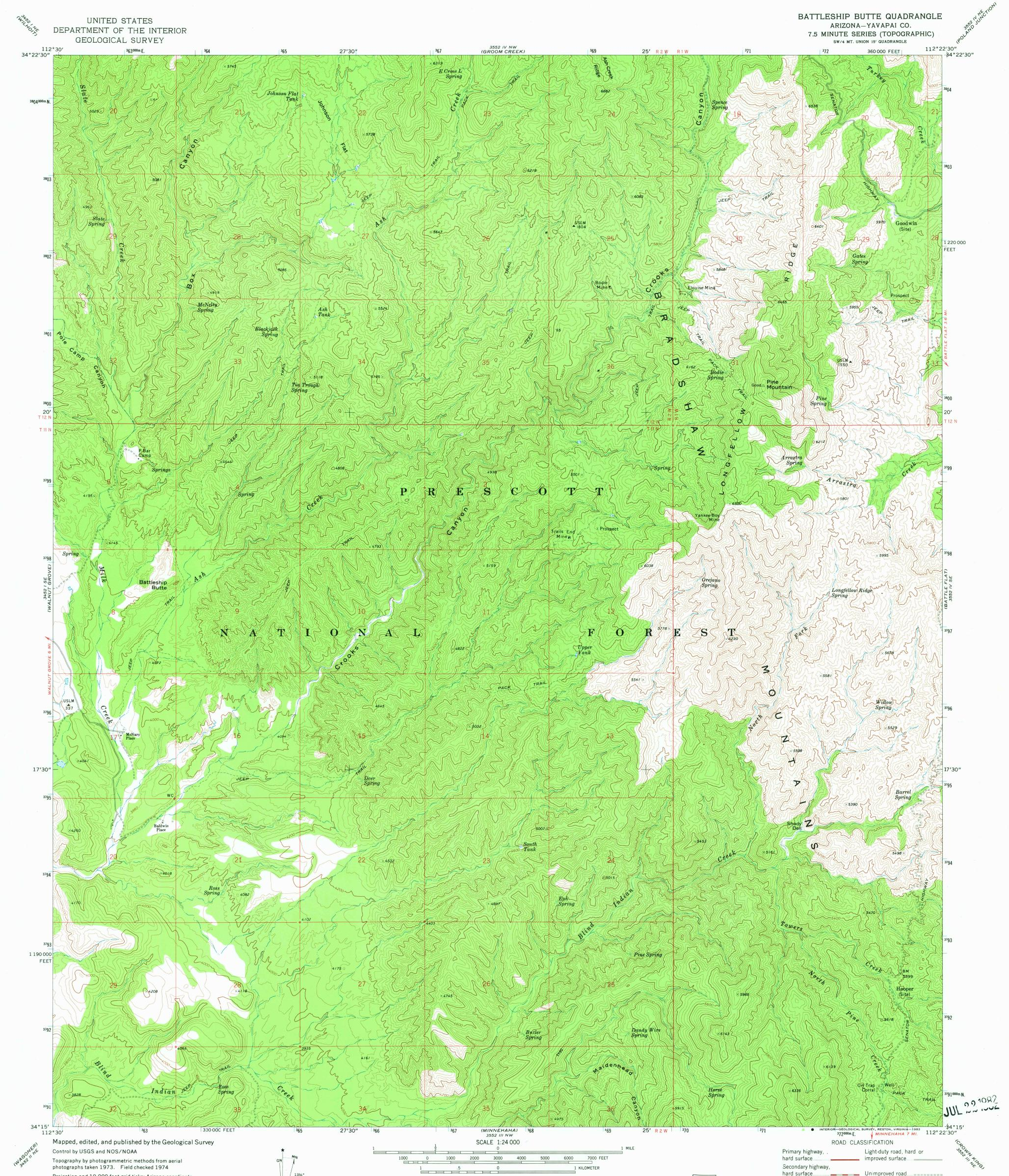
Projection and 10,000-foot grid ticks: Arizona coordinate system, central zone (transverse Mercator) 1000-meter Universal Transverse Mercator grid ticks, zone 12. shown in blue 1927 North American datum To place on the predicted North American Datum 1983 move the projection lines 1 meter north and 67 meters east as shown by dashed corner ticks Fine red dashed lines indicate selected fence lines Where omitted, land lines have not been established
